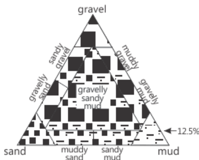
Fig. 6.2. Triangle diagram displaying the classification system for mud sand and gravel used. Modified from Melles and Kuhn (1993)
