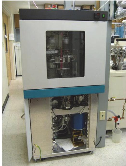
Figure 15: Figure 16: Picture of the Kiel-III preparation device in Oregon State University (McKay, J. 2015)
