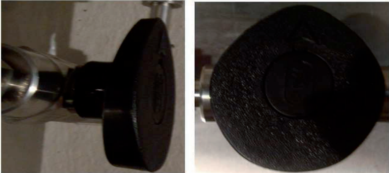
Figure 2-5: Shows Manual valve (V2 and V4)
