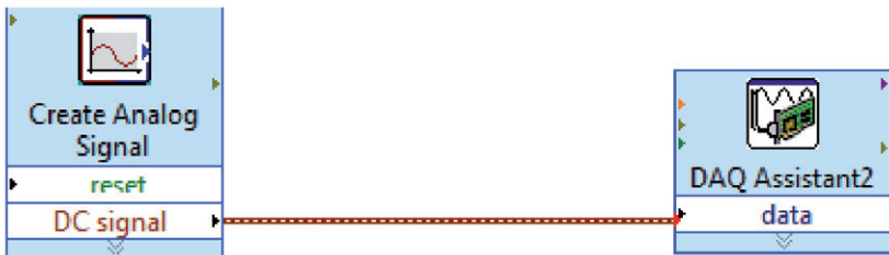
Figure 4-11: The code on the Block diagram for DC signal
