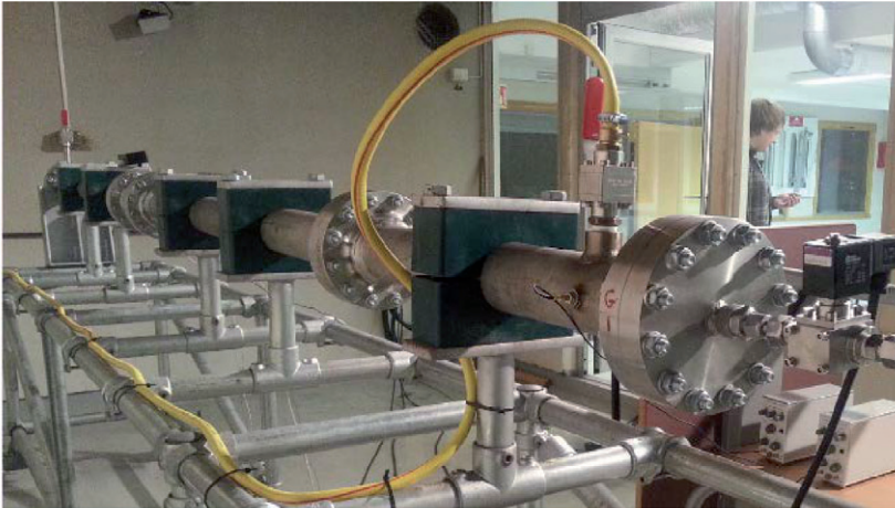
Figure 2-18: Driven section of the shock tube
