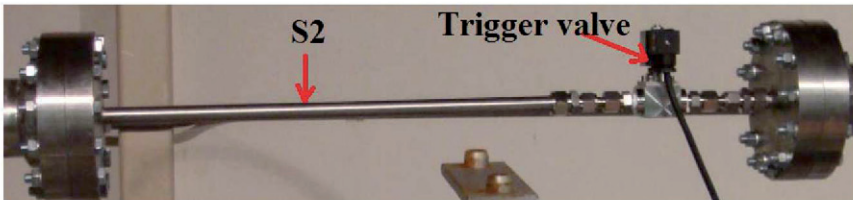
Figure 2-16: Subsection S2 of the driver section with trigger valve
