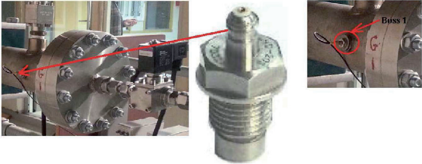
Figure 2-29: shows piezoelectric pressure transducer and boss 1
