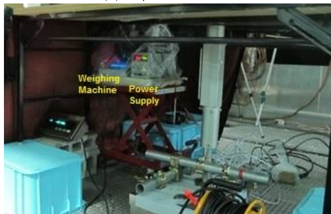
(c). Measurement setup under tunnel
