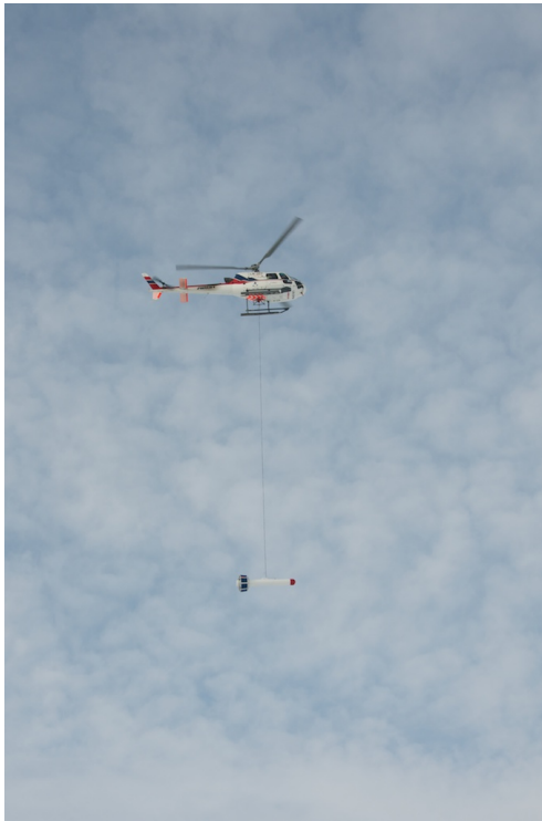
(a) Helicopter towing the EM-bird. Image courtesy of A. H. H. Renner.
