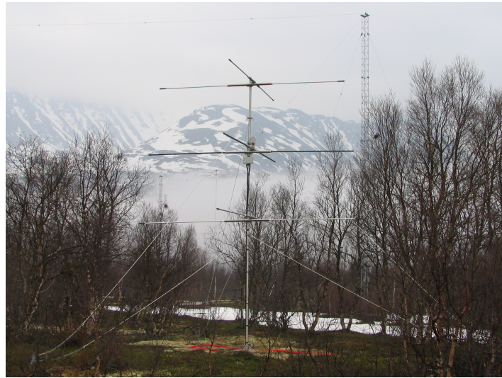
a) One of the six identical antennas which constitute the Nippon/Norway Tromsø Meteor Radar. Image credit: Chris Hall.
