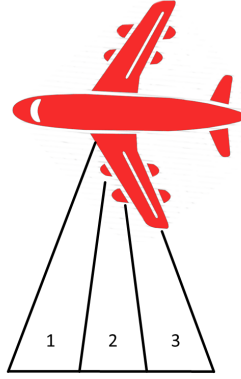
Figure 2.10: Splitting of the Synthetic Aperture Length in L=3 subsets.
