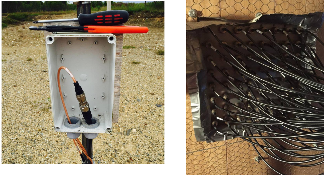
Figure 4.1: Figures showing the antenna box attached to each riometer antenna and the receiver rack in the riometer hut (Photo by: I. M. Larsen)
