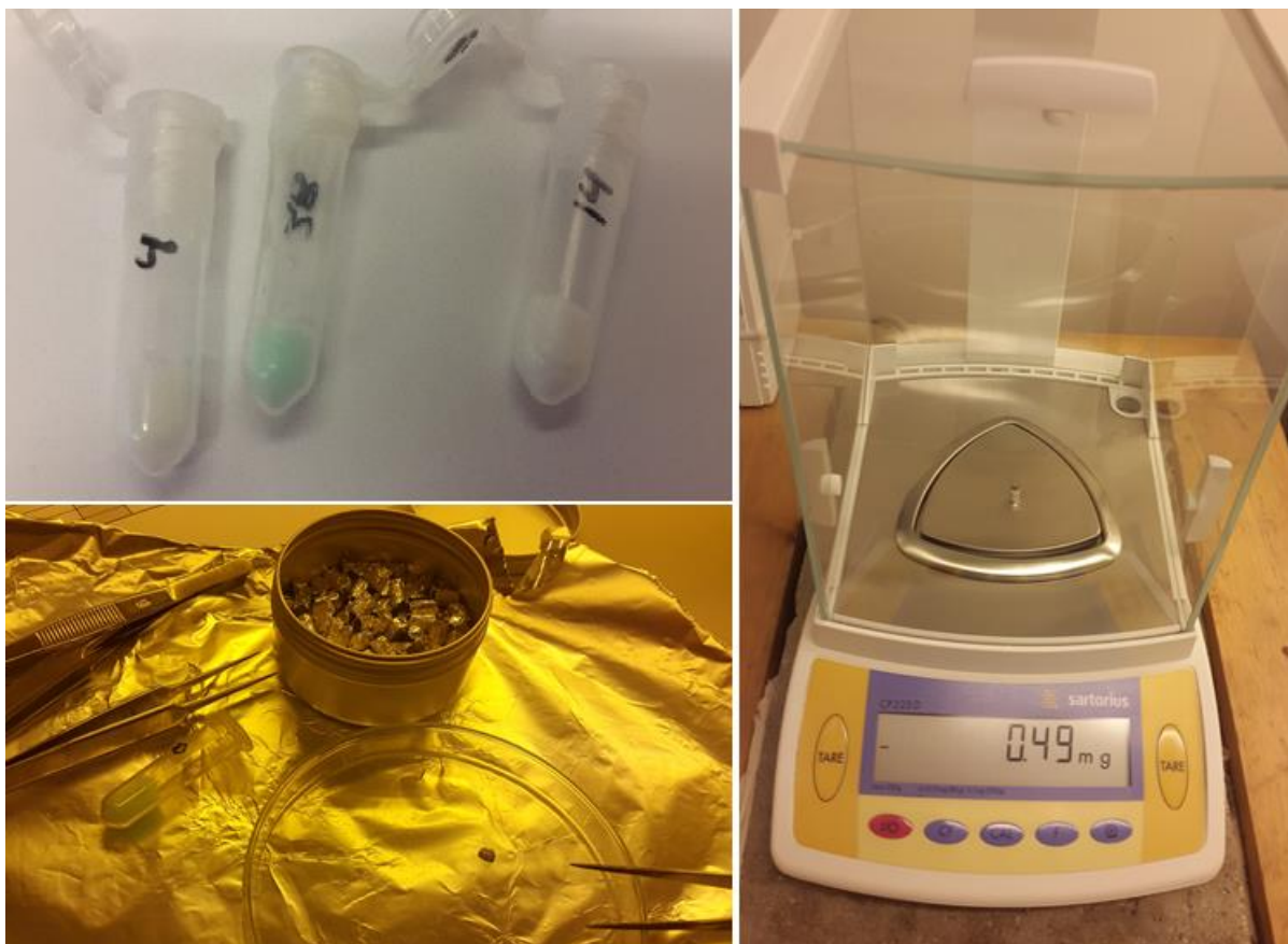
Fig 5. Collagen isolated from jaws of Icelandic arctic foxes (top left), illustration of samples weighing (right) and packing for stable isotope analysis (bottom left).
