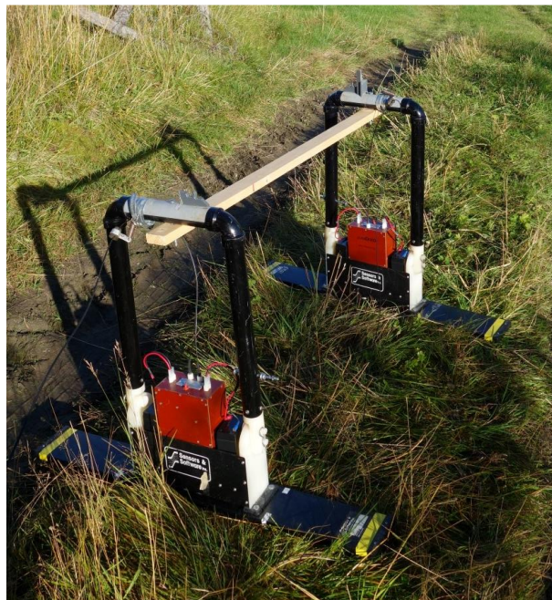
Figure 30: Photograph of the PulseEKKO™ IV GPR instrument used in this study. The antennae have a fixed position 1.0 m apart. Two people are required to operate the system: one person to move the GPR antennae; and one person to operate the computer.
