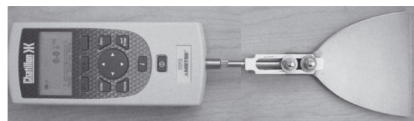
Figure 9. Blade hardness gauge, similar to the gauges used in this study. Modified from Borstad and McClung (2011).
