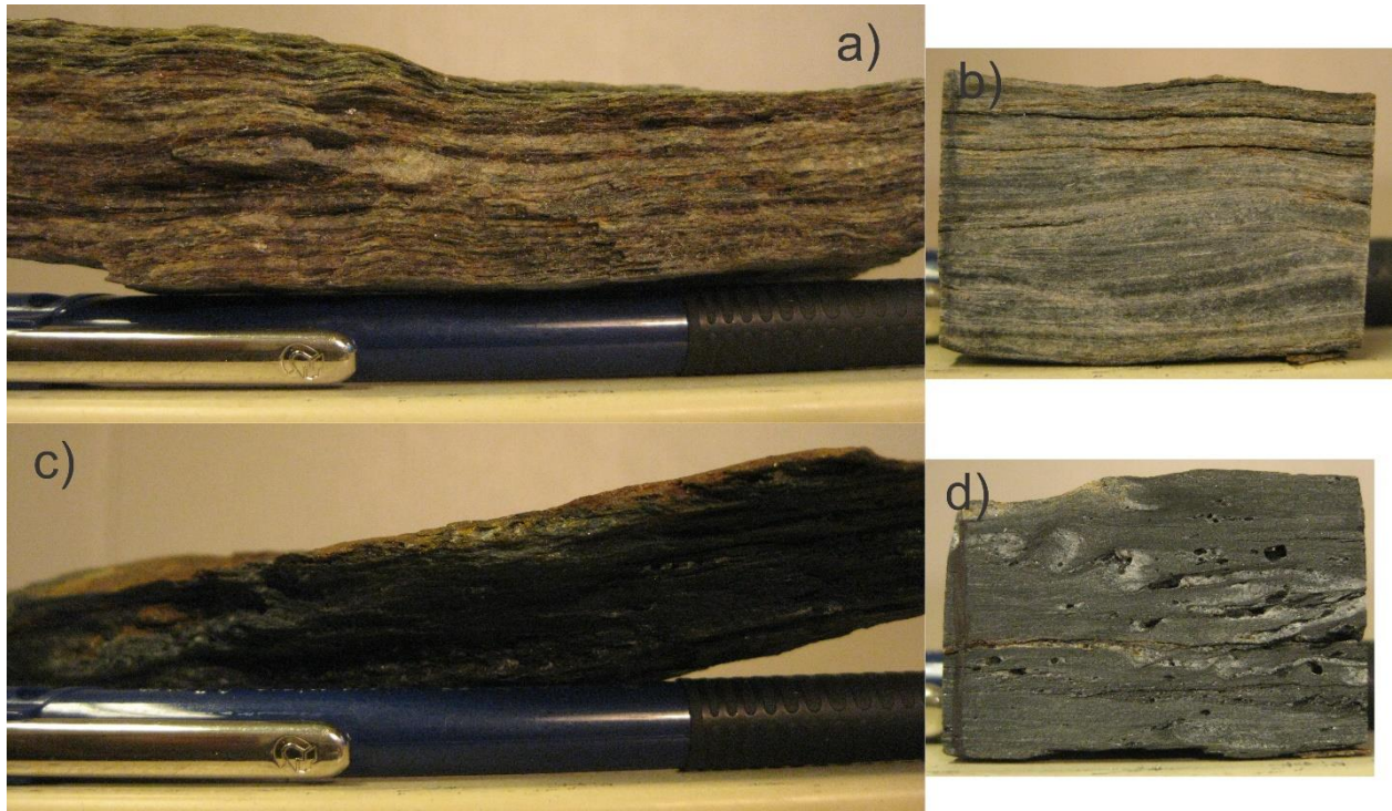
Figure 41 - Hand specimens of Phyllite. a) Fresh surface view of sample 4, showing slightly crenulated schistose foliation, with the foliation defined by thin bands of very fine-grained material. Bands of Quartz are also present. b) Cut view of sample 4, from thin section preparation. c) Fresh surface view of sample 6, displaying typical phyllitic graphite color. d) Cut view of sample 6, from thin section preparation. A dark, fine-grained matrix dominates, with lenses and clasts of Quartz also present.
