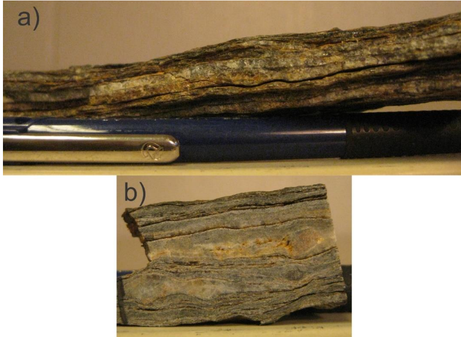
Figure 38 - Hand specimen of sample 3.1. a) Garnet Mica Schist displaying prominent Quartz bands, with thinner fine-grained bands rich in micas. Foliation is more schistose compared to the underlying gneiss. b) Cut view of sample 3.1, from thin section preparation.
