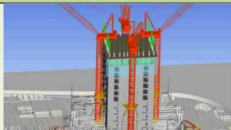
Figur 2.3-9: 4D Planning SH Tower ( Qing, 2012 ).
