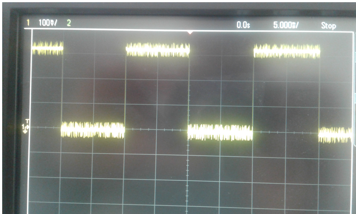
Figure 5.14: CA clock signal of 20 ms periodicity
