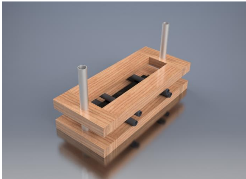
Figure 9: top view of the four-point test bench. The polyurethane specimen in the middle. The renders in fig. 8 and 9 are both modelled in Autodesk Inventor Professional 2017.
