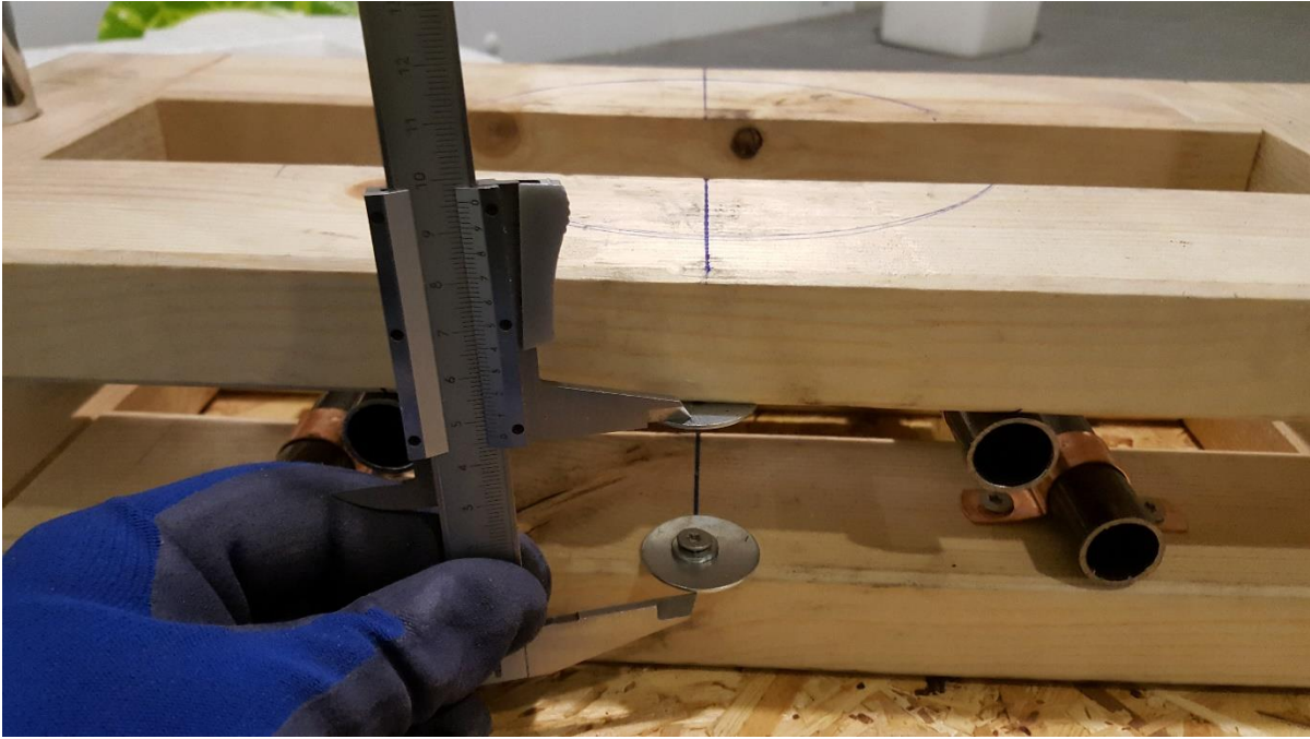
Figure 9: recording of displacement using a Vernier caliper. At this instant, the only load is from the upper frame alone. The middle of the frame is marked with a circle.
