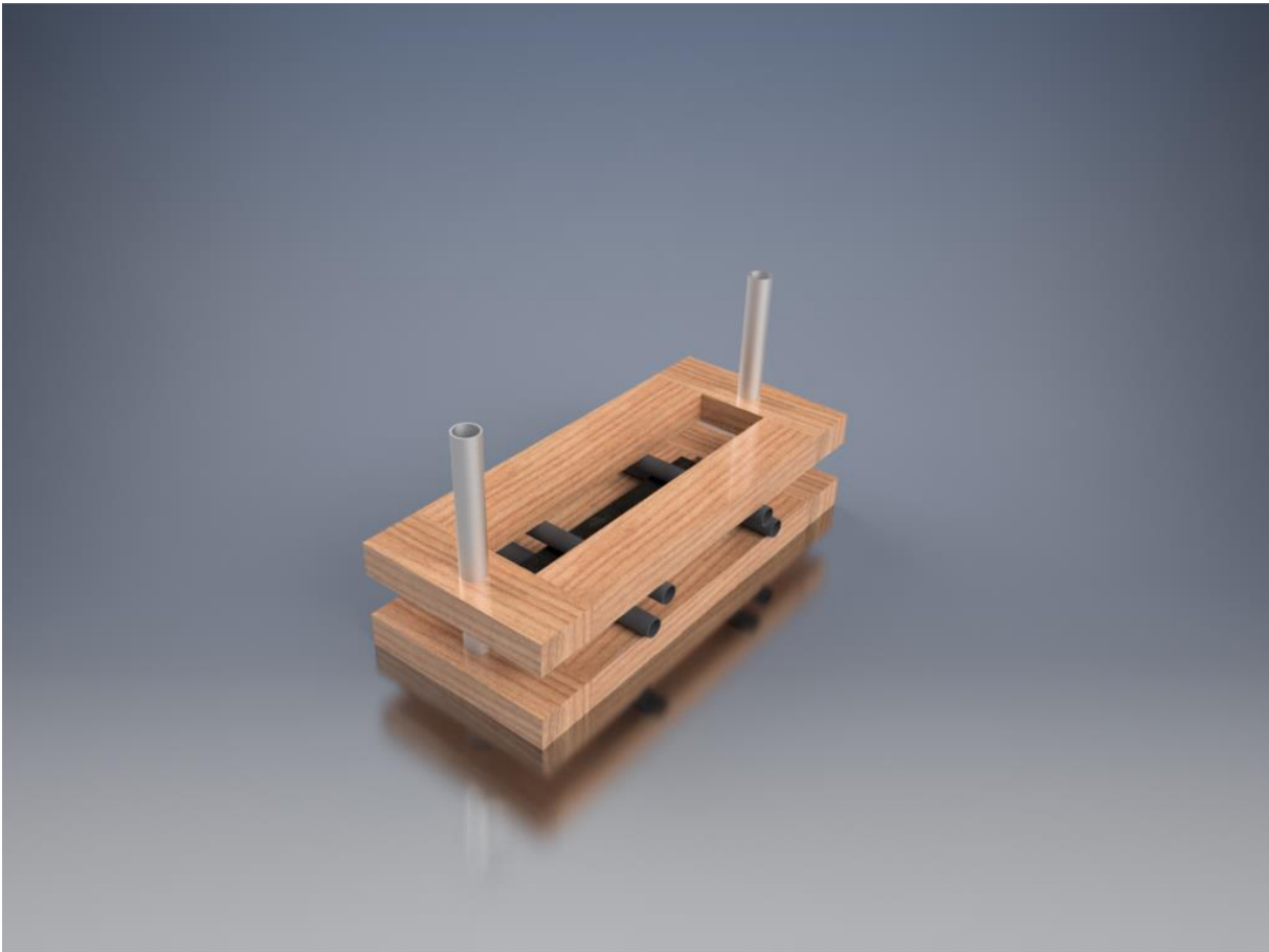
Figure 8: top view of the four-point test bench. The polyurethane specimen in the middle. The renders in fig. 5 and 6 are both modelled in Autodesk Inventor Professional 2017.
