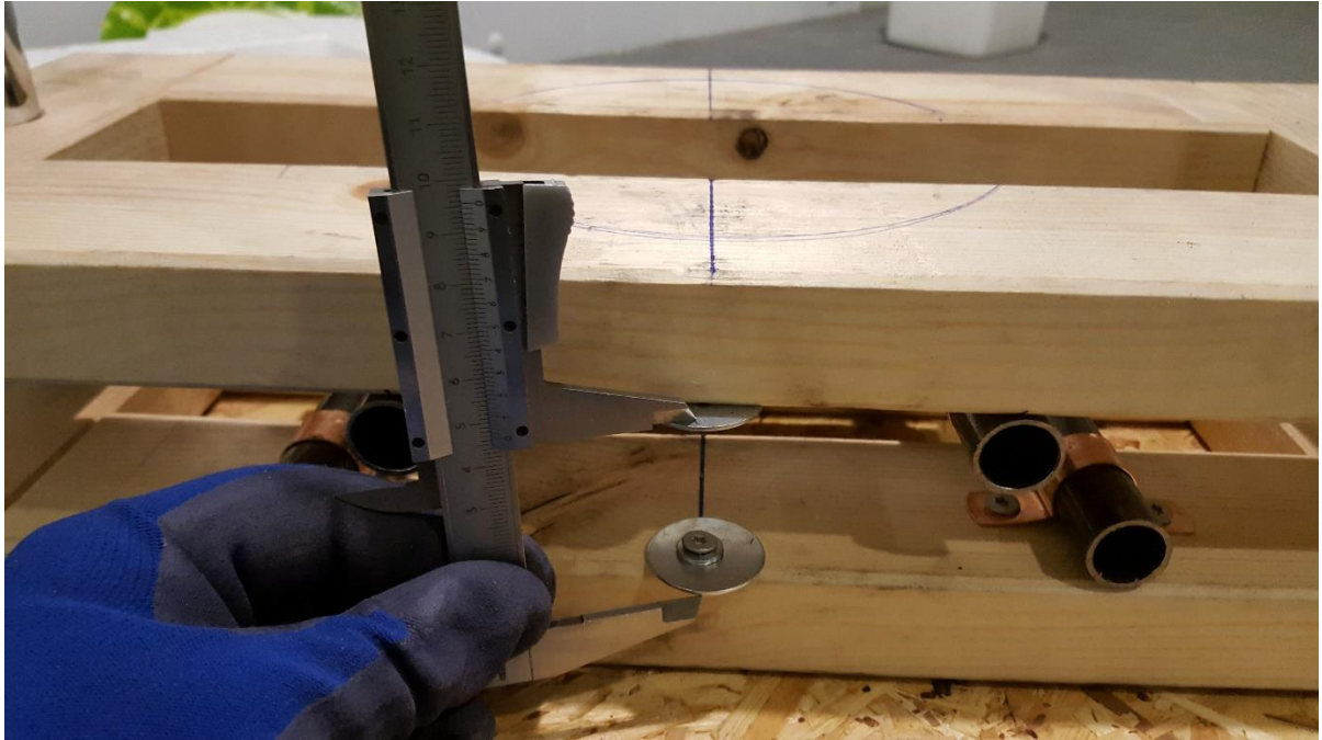
Figure 11: recording of displacement using a Vernier caliper. At this instant, the only load is from the upper frame alone. The middle of the frame is marked with a circle.
