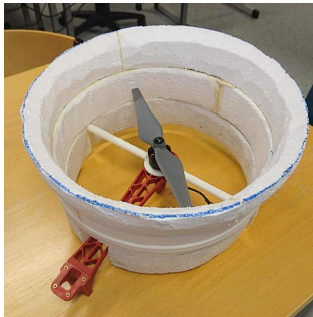
Figure 31. Prototype with drone arm and rotor.
