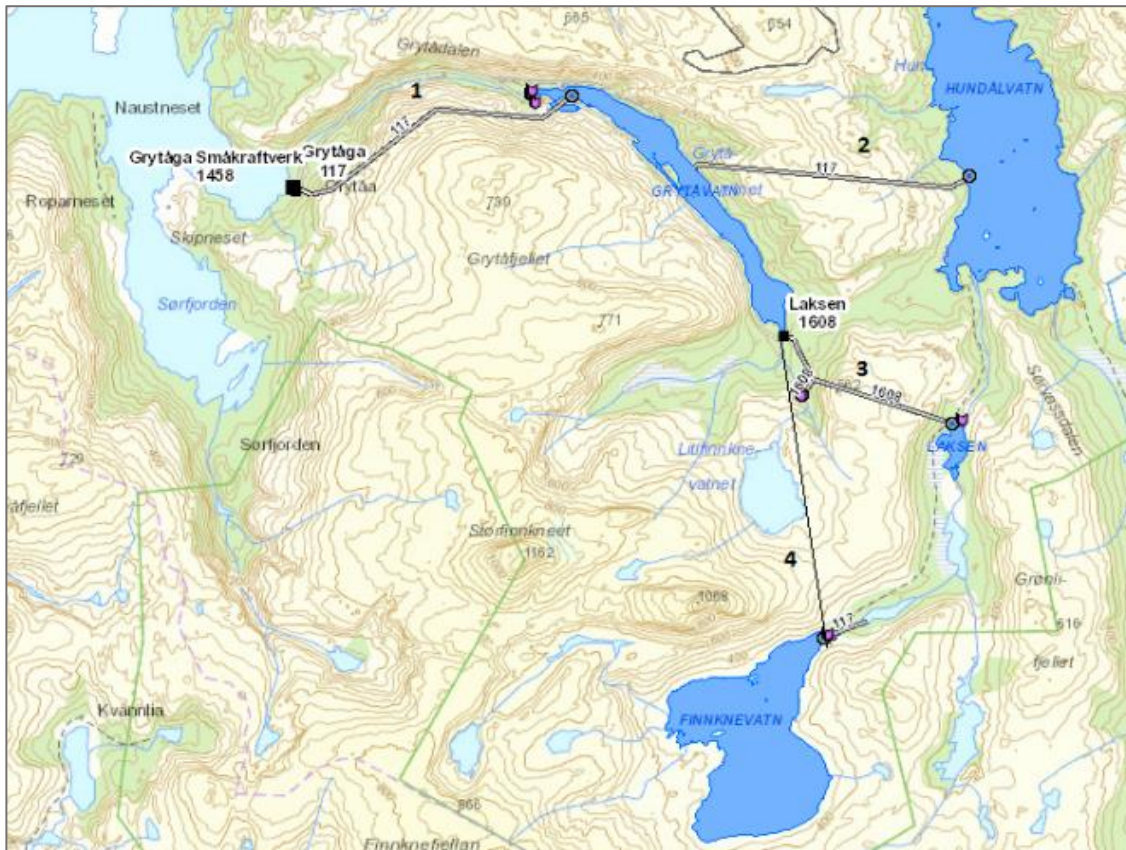
Figure 41: Grytåga PSH Project (atlas.nve.no, n.d.)
