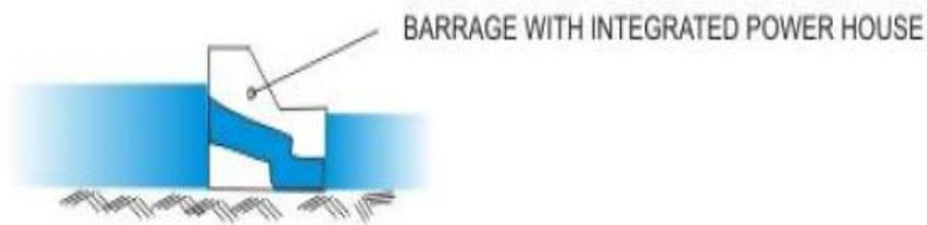
Figure 12: Run-of-river hydropower scheme. (SWR, 2008)
