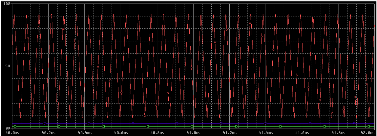
Figure 34: PWM signal with unipolar supplying op amps( DC voltage is minimum)
