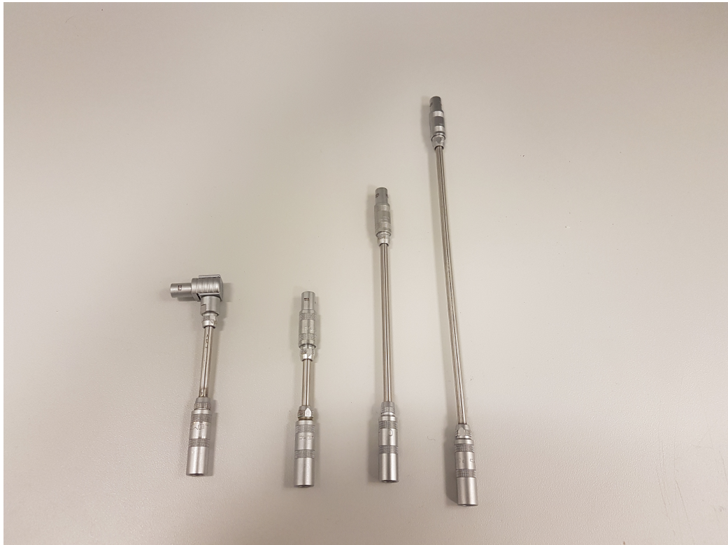
Figure 4.6: All the components that were made for this project to complement the Langmuir probe. From right to left: 90° "knee" component, 8 cm extension rod, 14 cm extension rod and 22 cm extension rod.
