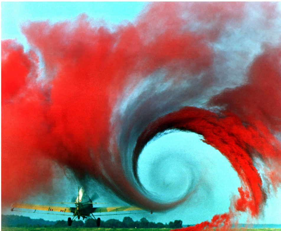
Figure 2.3: Wake vortex produced by the passage of an aircraft wing (NASA 1990)
