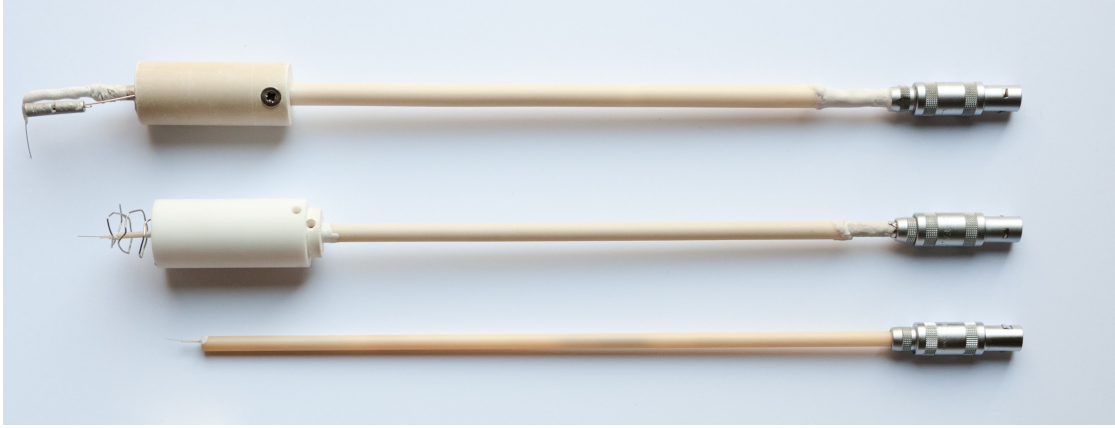
Figure 3.1: Examples of Langmuir probes used at UiT. The two upper probes are RF-compensated and the lower one is not compensated. The uppermost probe is the one used in this study.
