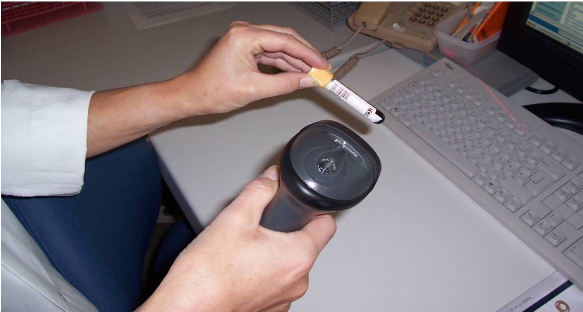
Figure 8: Illustrates how the bar code based sample tubes are scanned at the service provider (UNN).
