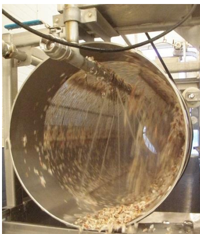
Figure 14 Tumbler for separating edible crab shell and meat
