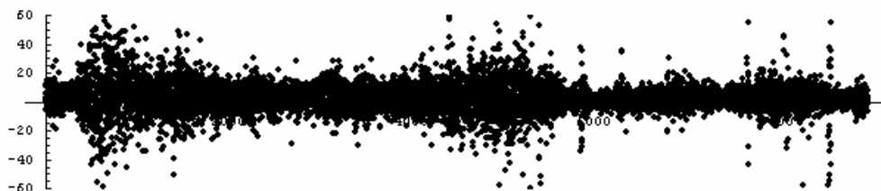
Figure 5.9→ Power vs samples plot without outliers. 13 of July 2004 from 07:59:58 to 09:00:00 and between 89.4 and 90.6 km altitude. 5 noise gates (8950 samples).
