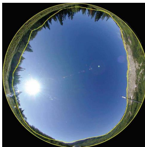
Figure 3-1: Hemispherical viewshed photo with calculated viewshed (yellow inner line). (Huang and Fu 2009)
