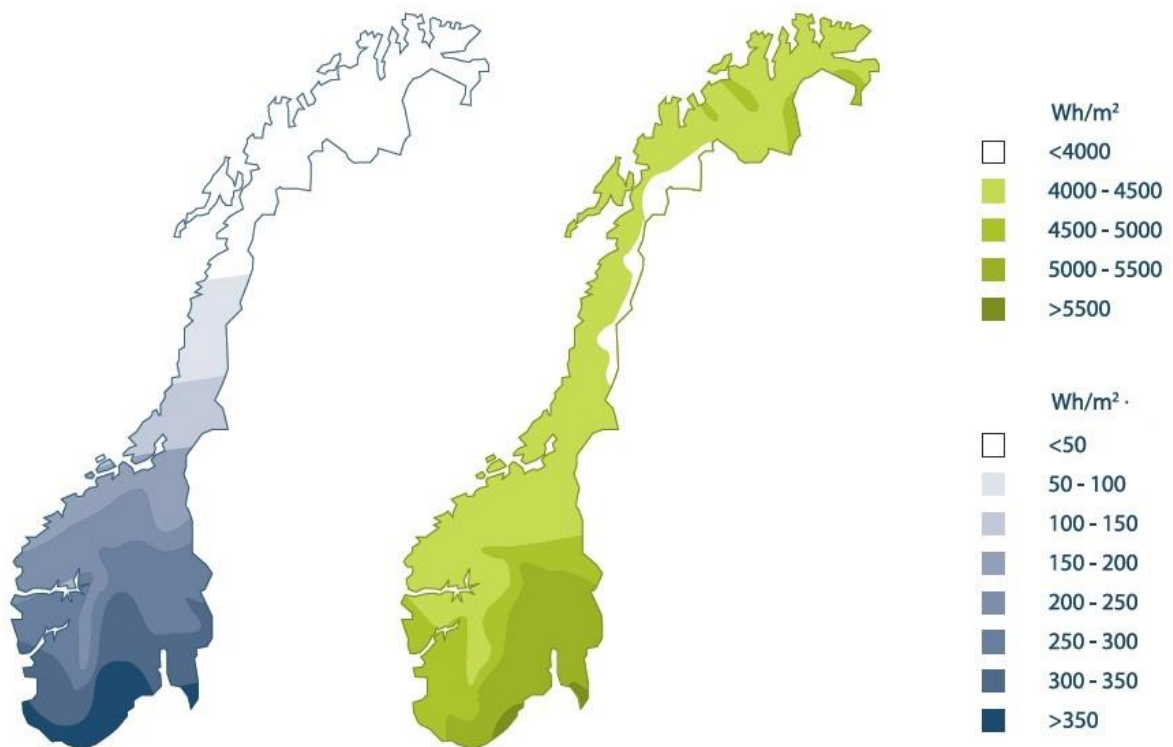
Figure 2-3: Global solar radiation per day for January (left map) and June (right map). Legend shows expected values of Wh/m 2 for each day, with the top legend being for June and the bottom for January. (Barstad 2016)
