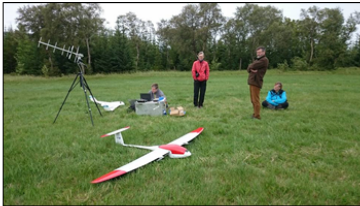
Figure 3.2: Crywing UAV and ground control systems.
