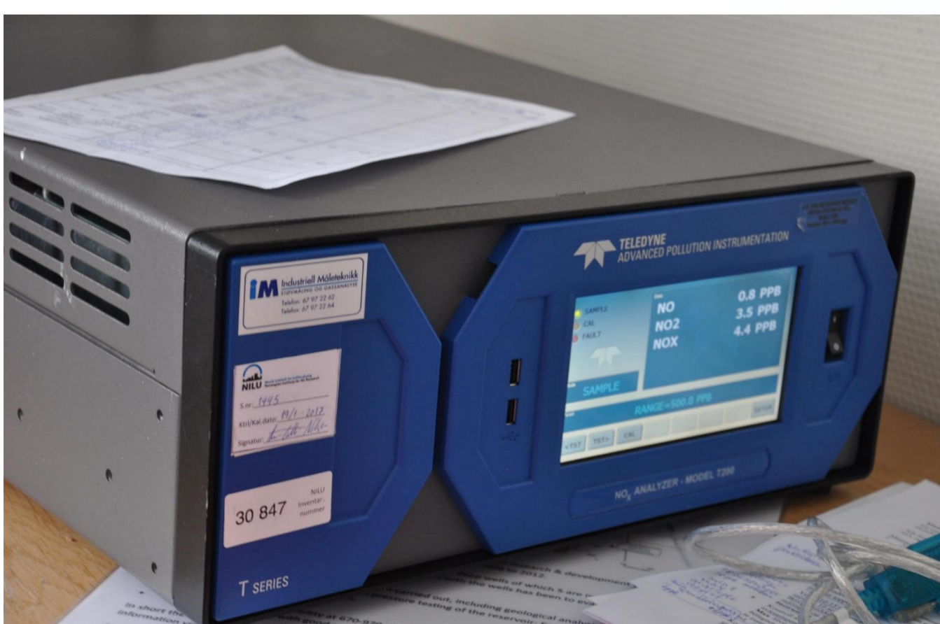
Figure 3 Chemiluminescence NO/NO 2 /NO x Analyzer (photo: Mark Hermanson)
