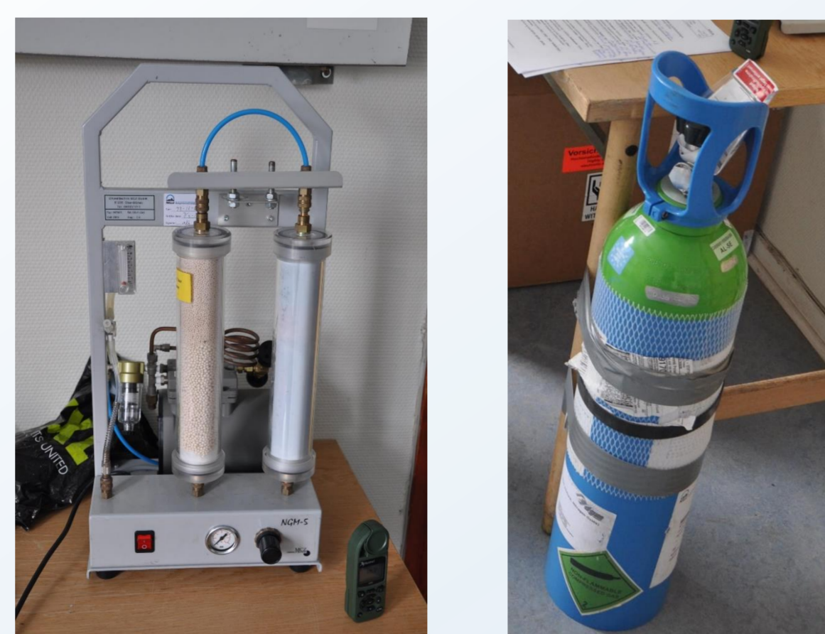
Figure 4 Equipment for weekly calibration of NO x monitor: a) zero air generator; b) gas cylinder with NO of known concentration (814 ppb) (photo: Mark Hermanson)
