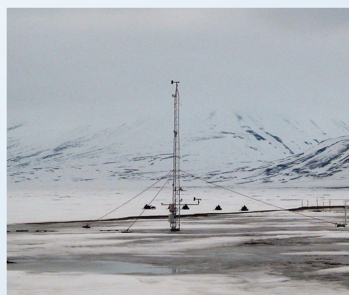
Figure 5 UNIS automatic weather station in Adventdalen
