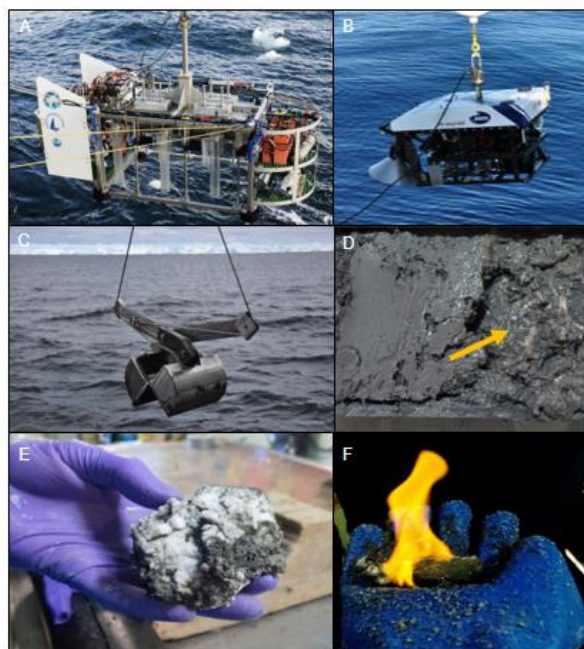
Figure 3: From upper left A) Tow-Cam, multicore and CTD (CAGE-MISO) used during CAGE 15-2 cruise. B) ROV K30 (NTNU) used for the cold seeps in the Barents Sea during CAGE 16-5. C) van Veen grab in open mode. D) Gas hydrates recovered in a gravity core. E) Ice crystals in the shape of gas hydrates. F) Burning methane gas from disassociating gas hydrates as it is recovered from the sampled cores.
