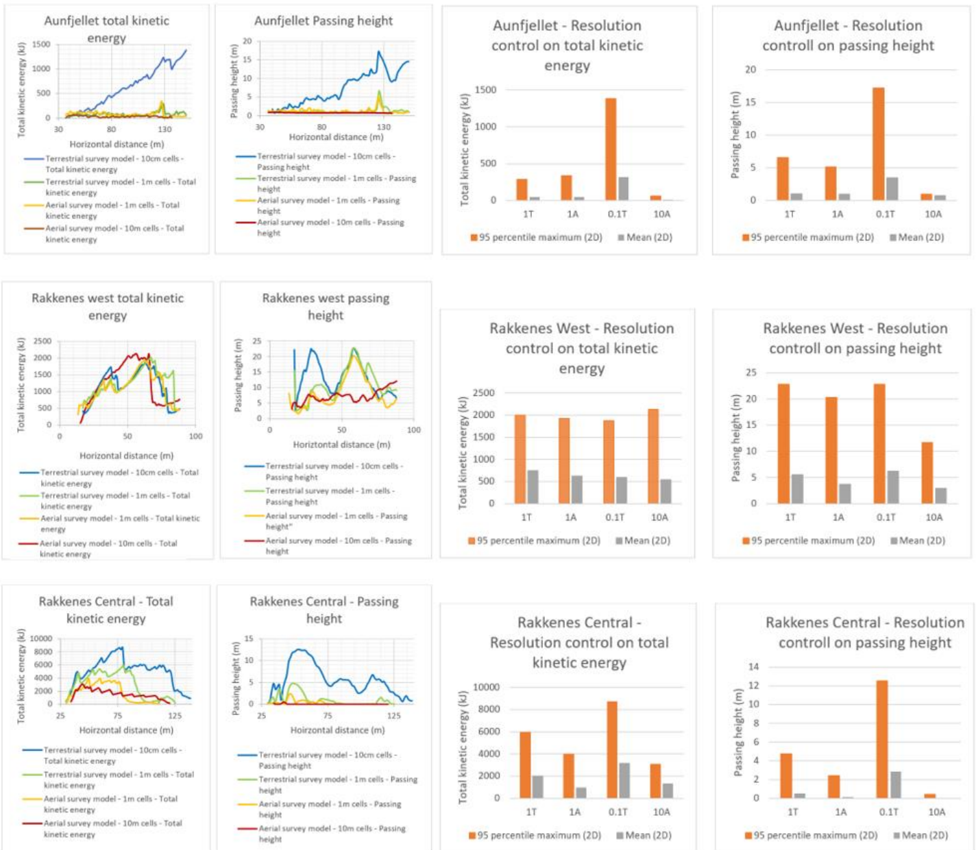
Figure 89: Summarizing statistics from all 2D simulations. Each row show results from a individual case area. Graphs are, from leftmost to rightmost column; ,max total kinetic energy as function of horizontal position, max passing height as function of horizontal position, summarizing statistics for total kinetic energy and summarizing statistics for passing height.
