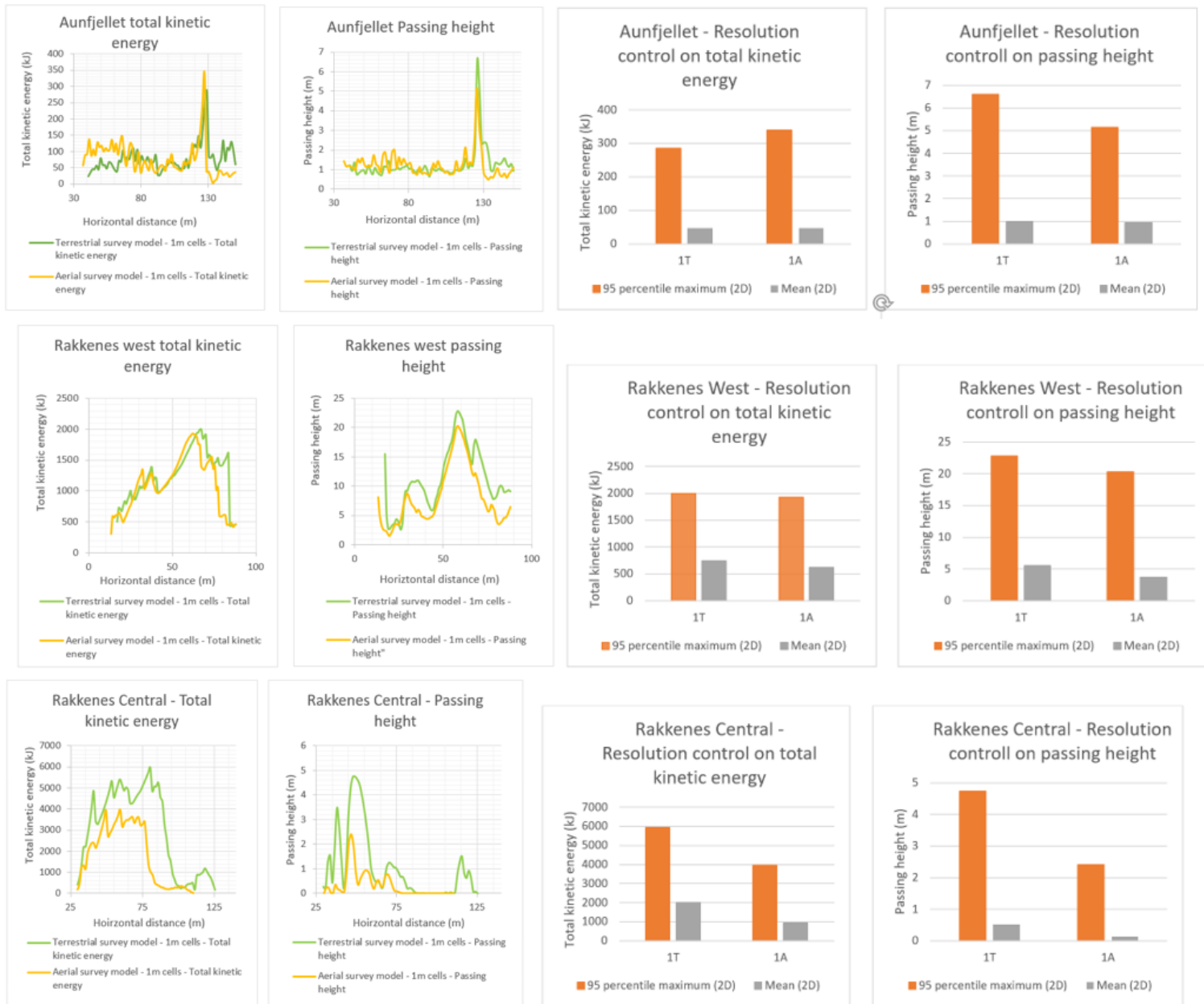
Figure 91: Summarizing statistics from all 2D simulations except the Revnestinden simulation. Each row show results from a individual case area. Graphs are, from leftmost to rightmost column; Max total kinetic energy as function of horizontal position, max passing height as function of horizontal position, summarizing statistics for total kinetic energy and summarizing statistics for passing height.
