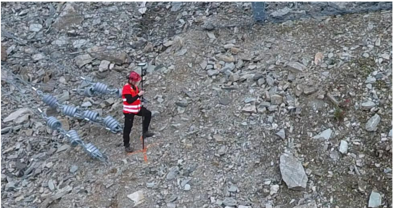
Figure 38: Geo-referencing ground control points in field.
