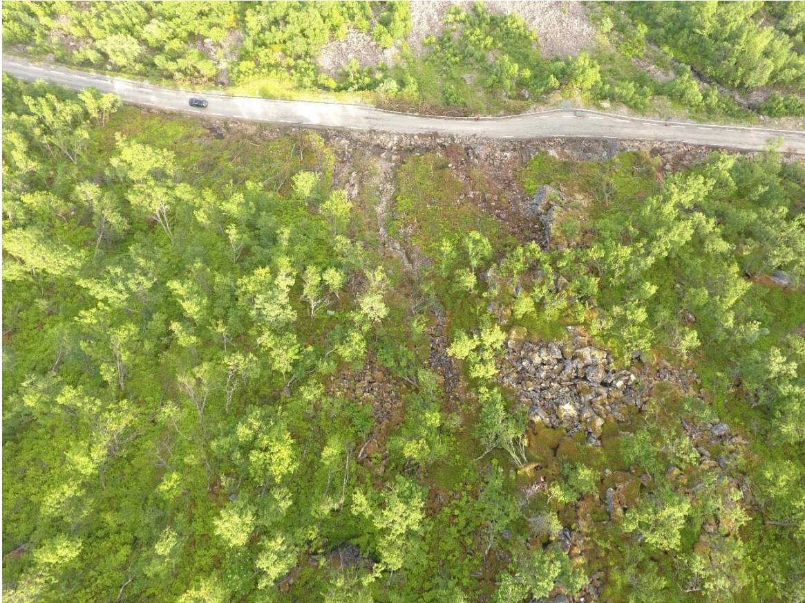
Figure 13: Run out area seen from above (drone photo), north is to the left. Notice unvegetated areas in the middle and above road, boulder concretion to the south and rocky outcrops above road.
