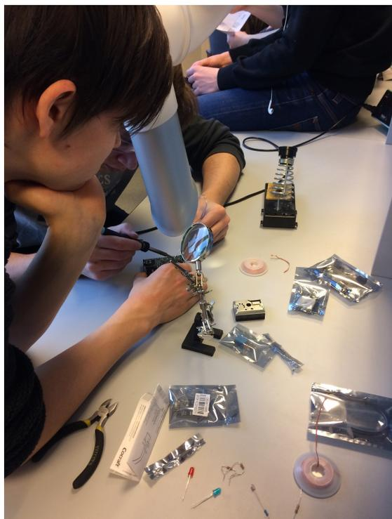
**Figure 2: Students soldering different components of the air quality sensor kits to the custom PCB Arduino Shield.**
