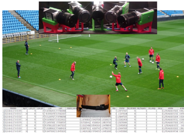
Figure 2.2: Illustration of the Bagadus system. The camera array captures video from the field. Video events can be extracted by performing queries on the ZXY database containing captured sensor data.
