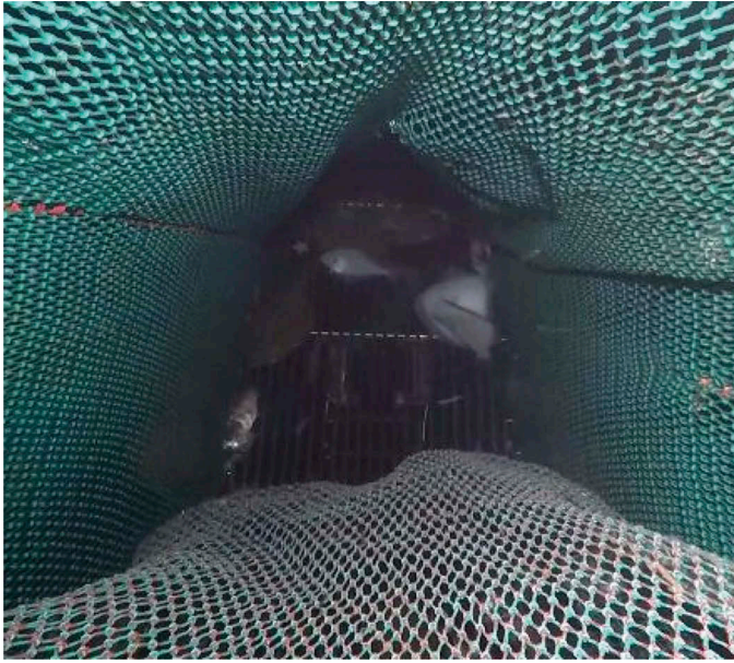
FIGURE 10. The Nordmøre grid during a normal tow with several American Plaice on and in the vicinity of the grid face.
