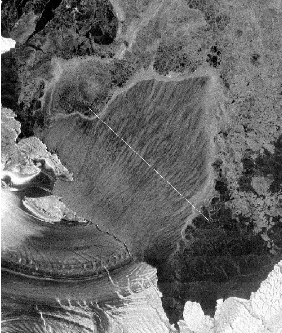
Figure 7.1: Example of grease ice in a SAR image. These can be seen as dark stripes perpendicular to the highlighted transect in the middle of the image. The slicks were validated from co-incident optical data. The image cover the Terra Nova Bay Polynya in Antarctica and is acquired by ALOS PALSAR (L-band) on 10 September in 2009. The image is provided as a processed joint photographic experts group (JPEG) file by Wolfgang Dierking through the ESA project ALO.3545.
