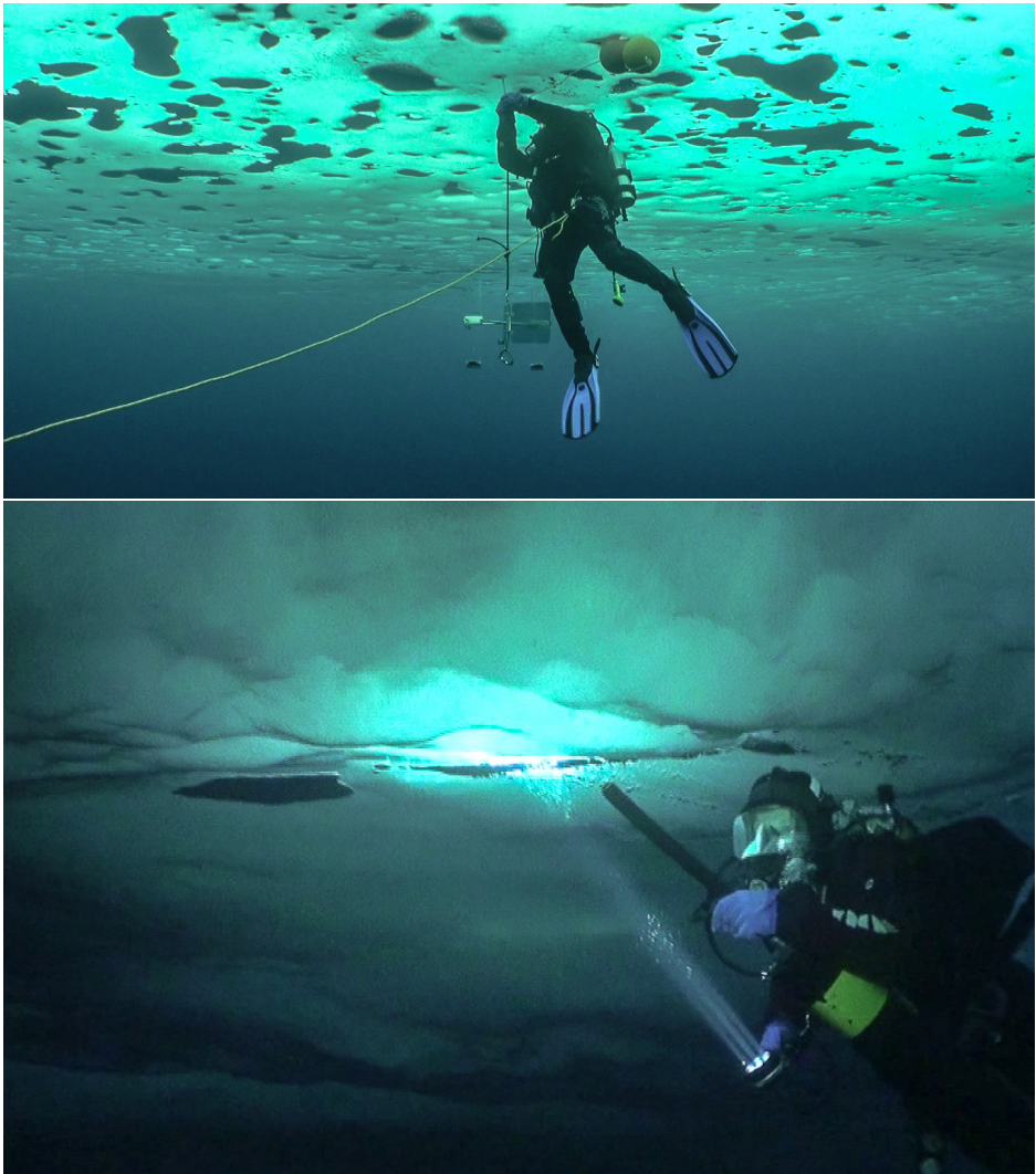
Figure 3.7: Underwater photographs showing the interface between sea ice and sea water. The roughness of the interface may play an important role to microwave scattering for wavelengths that can penetrate through the sea ice. The images are taken during the N-ICE 2015 campaign. The top and bottom image are from the 10th and 18th May, respectively. In general, little is however known about typical roughness conditions of the ice-water interface. Image courtesy: Haakon Hop, norwegian polar institute (NPI)
