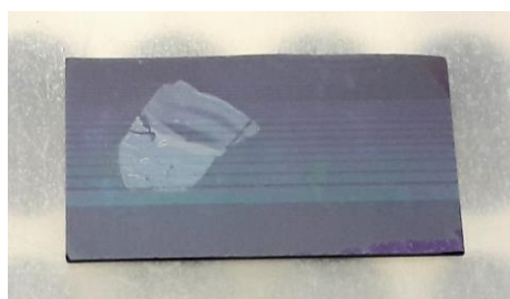
Figure 3.20. Human liver FFPE tissue section on top of a photonic chip. The straight lines on chip correspond to various waveguide widths for imaging. Chip size approx. 2.5 x 1.5 cm.
