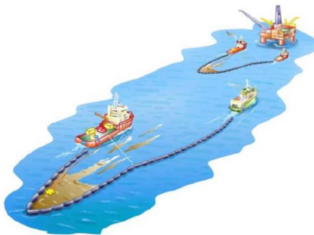
Figure 4.1 Open-ocean mechanical recovery systems (source: NOFO)
