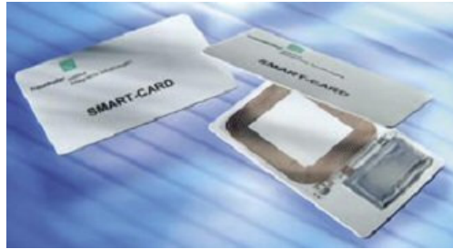
Figure 30: Smart-card with a wireless battery charge system [69].
