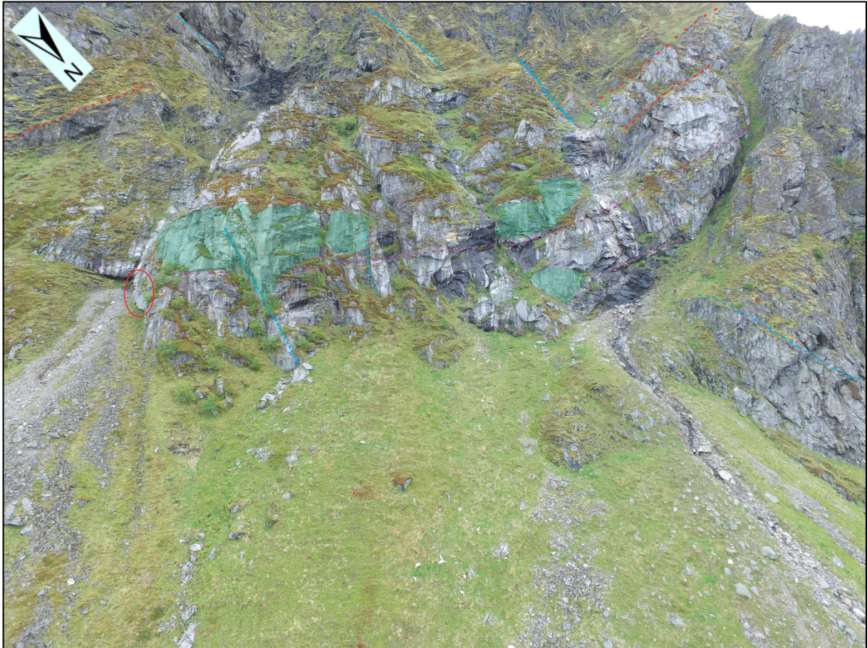
Fig. 43 Outcrop photo of the steep mountain side of Slettind, with close-up view of location 2 (see fig. 44). The light-colored meta-psammitic schists/gneisses have well-defined composite foliation dipping gently to the SW (left in photo) and is apparently folded by open folds yielding variable dips (and strike directions). Brittle J2-fractures/joints (red-colored stippled lines) are low- to moderate angle and subparallel to the gneiss foliation. Red dotted lines follows the N-S striking joint set J1, that here changes slightly in dip. Blue dotted lines follow the low angle north dipping J2 and green areas represents the planes of J3. Photo taken with UAV.
