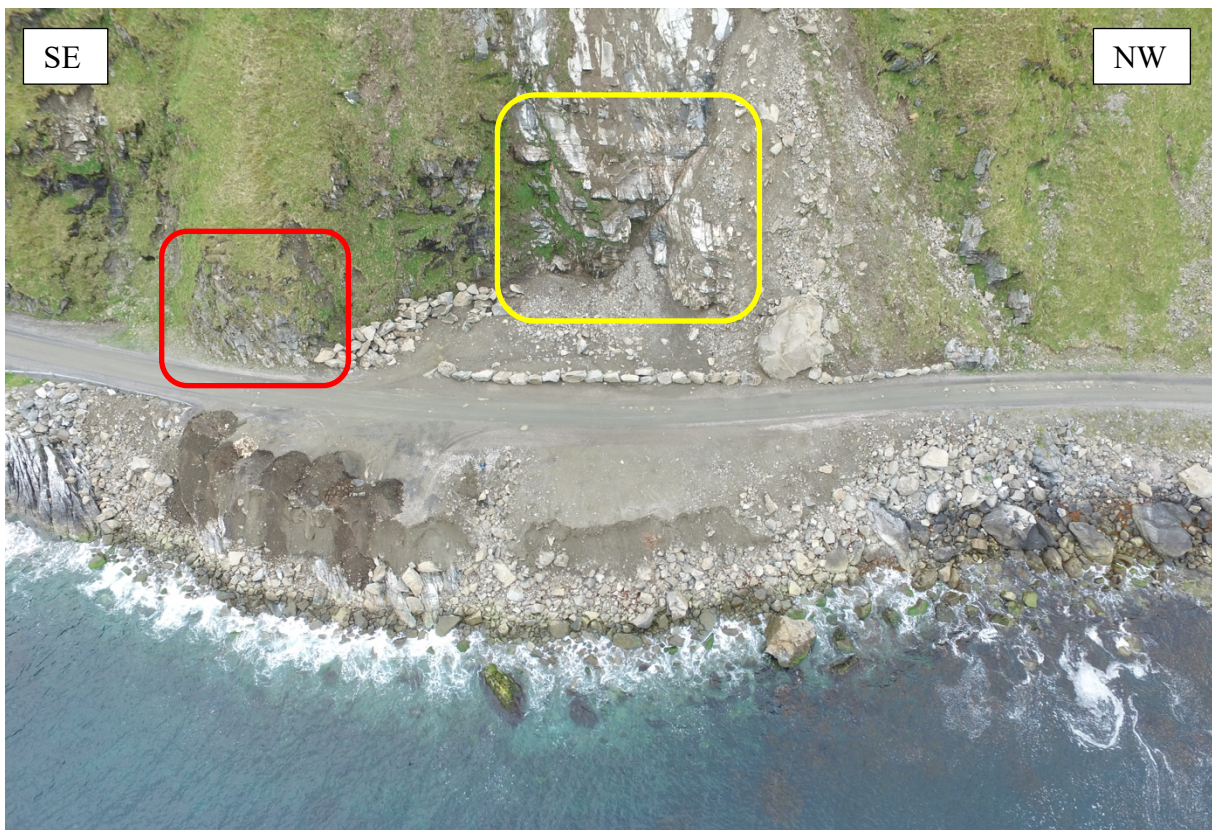
Fig. 38 Picture showing an overview of the first outcrops. Location 1.a is within the red box and location 1.b within yellow box. Joint sets J1, J3 and J2 are visible in the picture. Picture taken with the UAV
