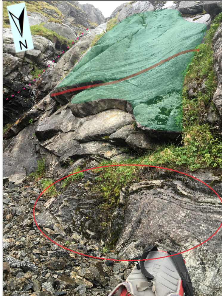
Fig. 44 Folds and fold hinges were found high near a larger weak structure. The overhanging joints follows the foliation orientation.
