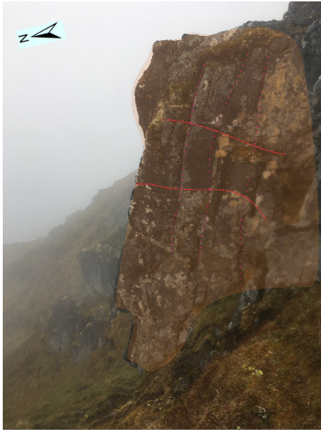
Fig. 49 Pictures from the summit ridge looking southeast. Clean vertical planes along the side of the funnels (marked as a red surface) are split by vertical, evenly distributed NW-SE striking joints and a horizontal joint set (red lines) creating an orthogonal blocky structure.
