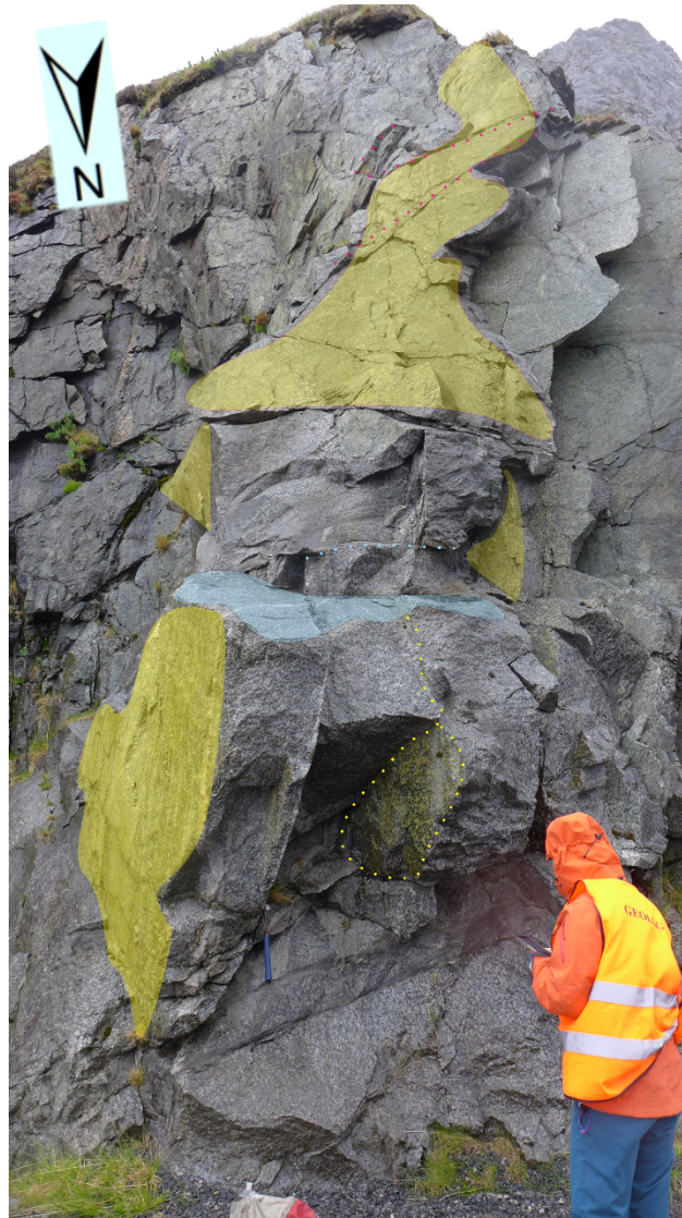
Fig. 47 Outcrop of location 3 shows surfaces marked with yellow (J1) and blue (J2). Yellow dotted line encircles a N-S striking surface where the greenish color is from epidote stains. Blue dotted lines follows the joints of J2. Note the ductile deformation band below the hammer.
