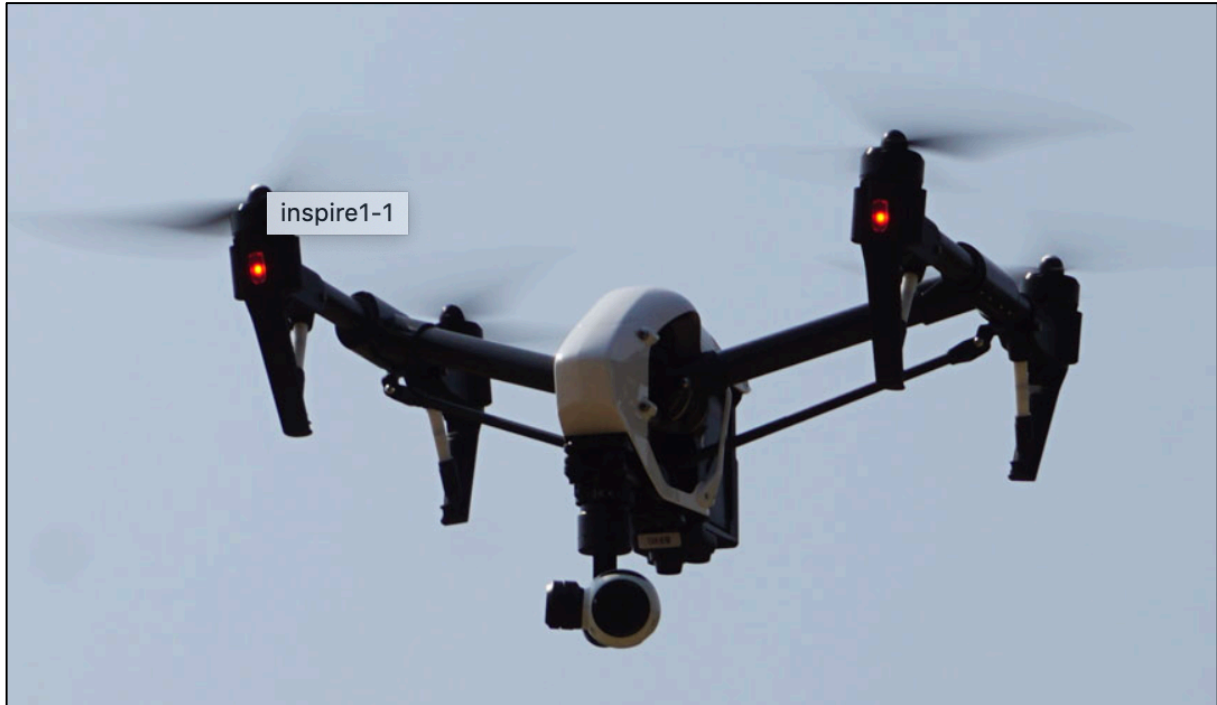
Fig. 26 The DJI Inspire1 is a large drone constructed for being stable at high altitude and taking good quality images. Picture from Drone business directory (2014).
