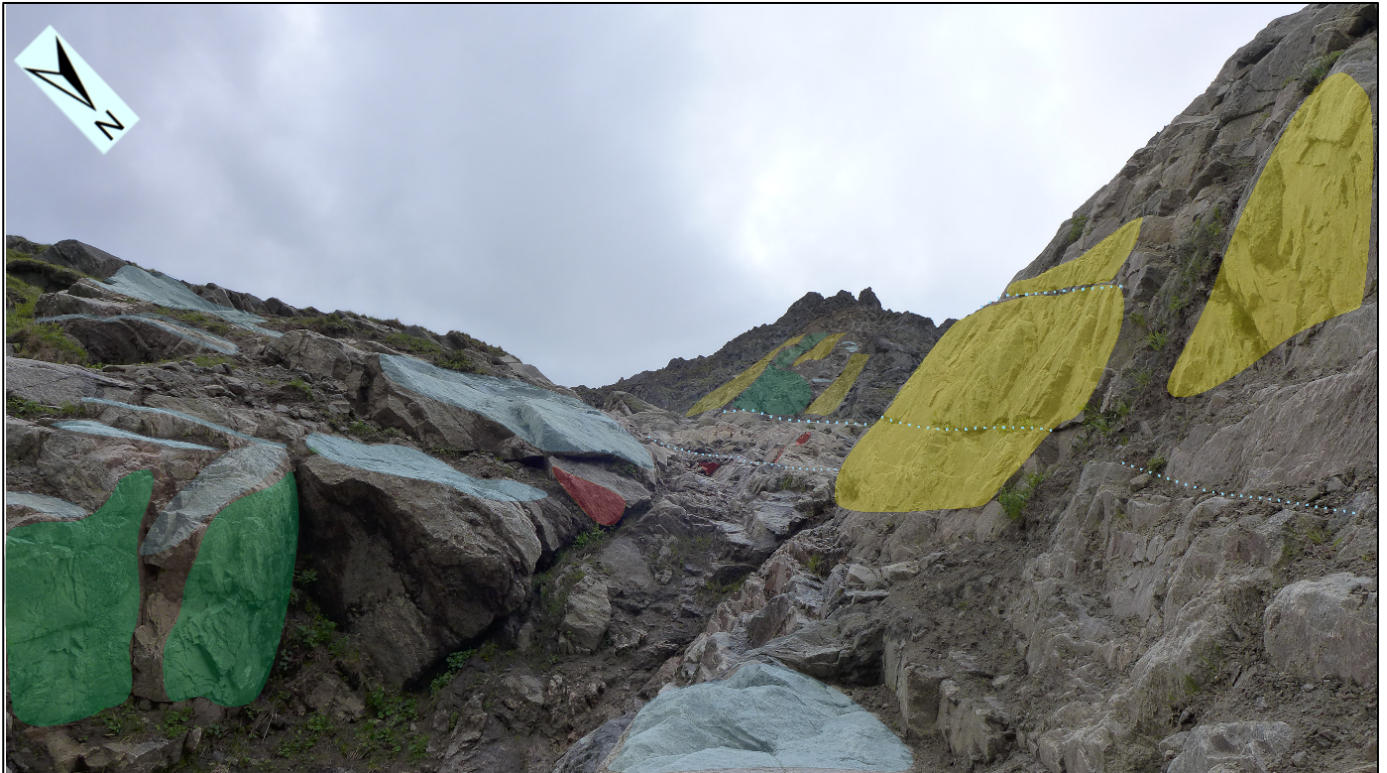
Fig. 41 Outcrop 1.b looking up towards the source area. Yellow surfaces are the steep north-south striking planes of J1, blue J2, green J3, and red the foliation. Dotted lines show joint sets of J2. From location 1.2 the source area 2011/17 and surfaces are easily identified and comparable.
