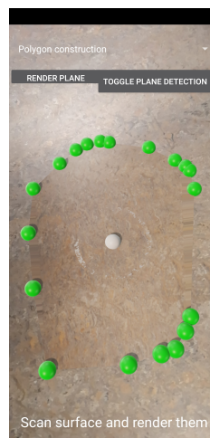
Figure 4.4: A polygon being created from triangles. Each triangle are made up by two green spheres on the outer edge and the plane's white centroid.
