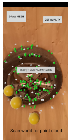
(a) A point cloud from a car tire captured indoors with 43.3 lx as seen at a distance of \sim 50 cm.
