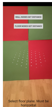
Figure 5.8: The vertically aligned paper sheets and the plane detection spotlight misinterpreting the surface to be horizontal. The wooden surface below surface D is a horizontal floor.
