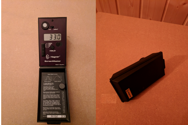
Figure 5.2: A lux-meter used to read illuminance of a surface. For the sake of completeness, we demonstrate how it reads illuminance in the image to the left. An example reading of 33.0 lx is shown.
