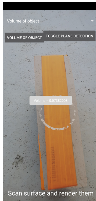
Figure 5.13: The uppermost horizontal polygon of the object. In addition, the volume in cubic meters is displayed.
