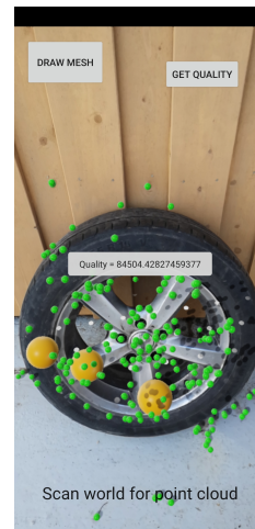
(b) A point cloud from the same car tire captured outdoors with 4590 lx as seen at a distance of \sim 50 cm.
