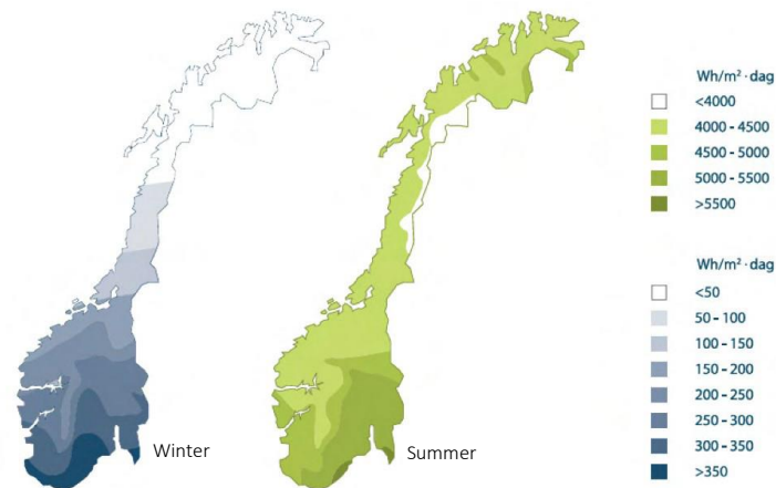
Figure 1. Solar irradiation on a horizontal surface in Norway for winter and summer. (Hagos, et al., 2014)
