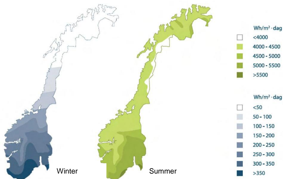
Figure 4. Solar irradiation on a horizontal surface in Norway for winter and summer. (Hagos, et al., 2014)
