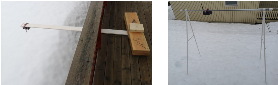
(a) Plank deployment of the IoT device. (b) Clothesline deployment of the IoT device.
