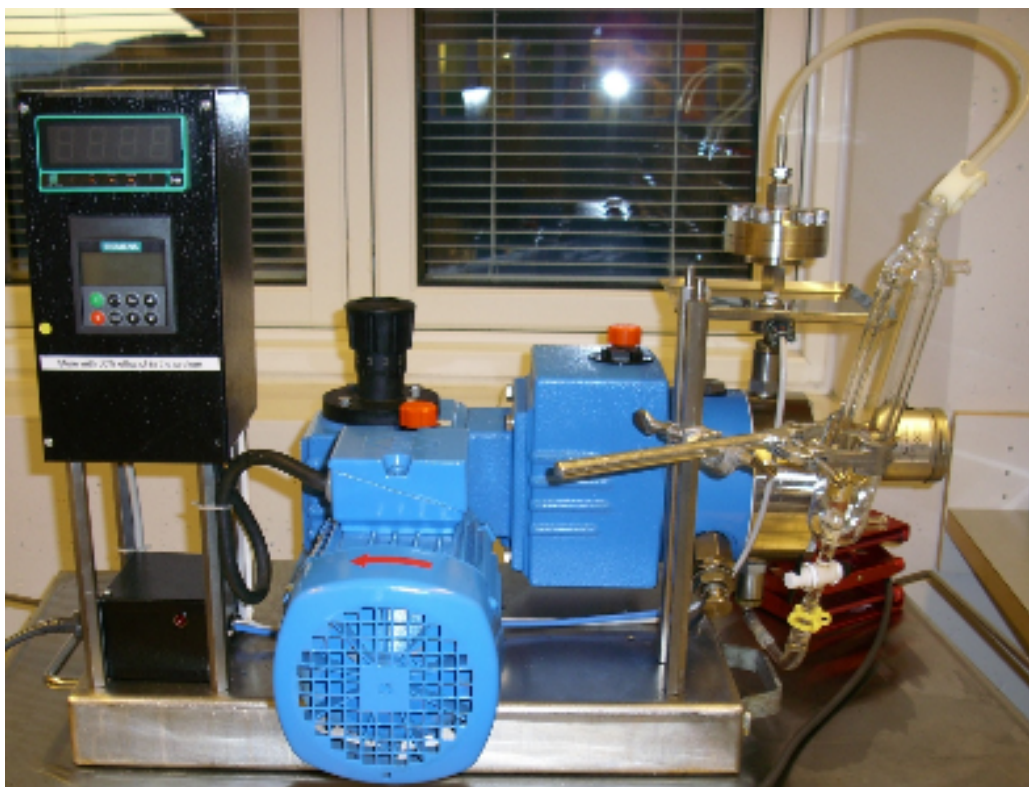
Figure 5.4.1: The custom made extruder
