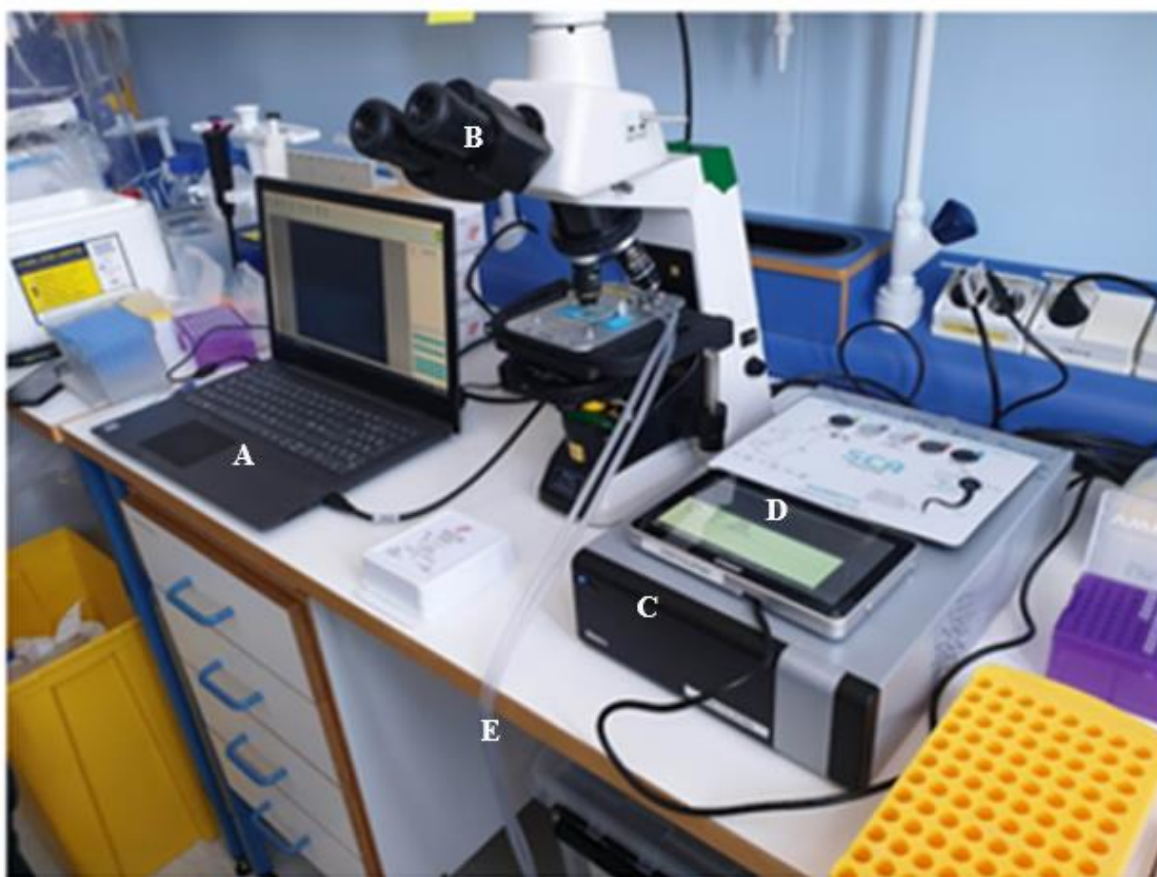
Figure 8. Experimental setup for sperm quality check using CASA system. (A) Laptop equipped with software analyzer. (B) A phase contrast microscope (Nikon E-200, Nikon, Tokyo, Japan) with x 10 negative phase contrast objective. (C) CASA system. (D) Temperature regulator cooling device. (E) Hose supplying chilled water to the slide.
