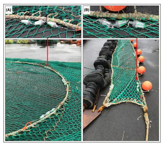
**Figure 16**. Images of an LEDs attached **(A)** near the center of the trawl headrope on the starboard side and **(B)** along the wing tip on the port side, and their orientations. Source: Paper V.
