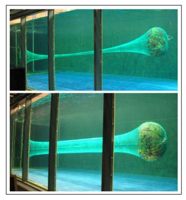
**Figure 5**. Flume tank model of a diamond mesh configuration codend (top image) and T90 mesh configuration codend (bottom image) stretched under longitudinal tension. Source: Digre et al. (2010).
