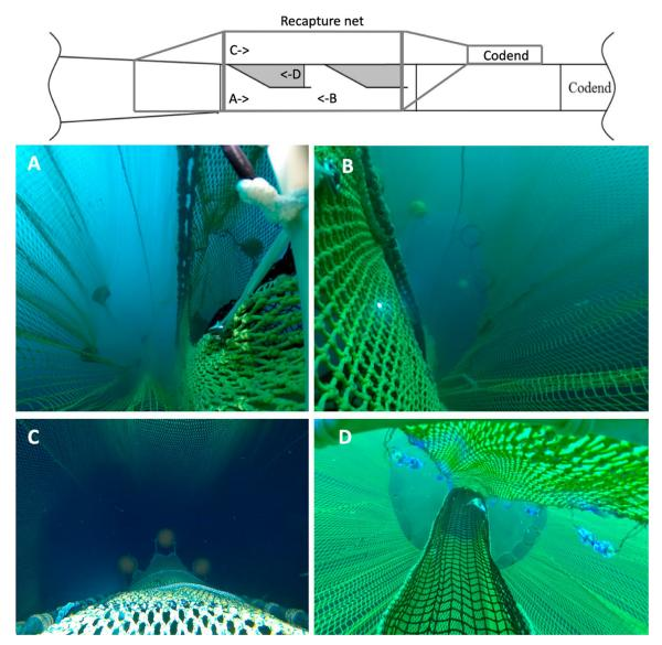
Fig. 3. Schematic diagram and images under ambient light examining the recapture net over the BRD in Experiment 2. Port-side aft view from outside of the BRD (image A); starboard-side forward view from outside of the BRD (image B); top panel aft view from outside the BRD (image C); forward view of the forward set of escape windows from within the BRD (image D). Note: diagram not to scale.
