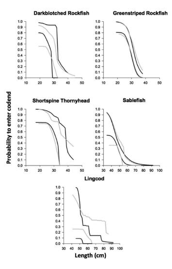
FIGURE 8. Comparison of the 95% confidence interval limits for the sizeselection curves quantifying a fish's probability of entering the cod end of a trawl equipped with one of two bycatch reduction devices (BRD-1 and BRD-2), as estimated for five roundfishes (length = cm TL for Shortspine Thornyheads and Lingcod; cm FL for all others). Solid black lines represent BRD-1 (6.4-  $\times$  25.4-cm grid size); solid gray lines represent BRD-2 (6.4-  $\times$ 30.5-cm grid size).
