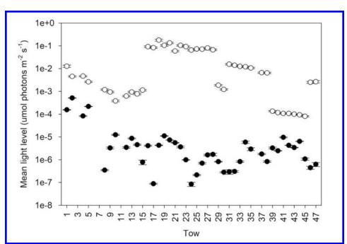
Figure 3. Mean light level measured at the center of the fishing line for the unilluminated trawl (closed circles) and illuminated trawl (open circles) per tow.  $\pm$  bars are standard errors (n = 50 measurements per net per tow).
