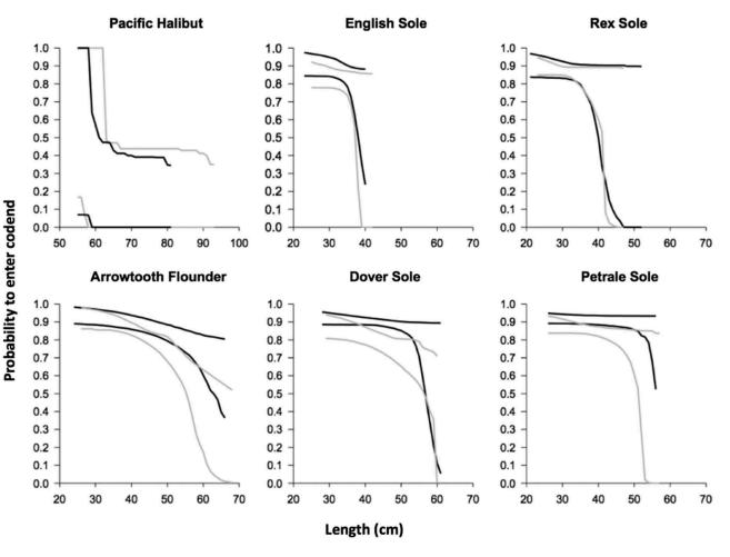
FIGURE 5. Comparison of the 95% confidence interval limits for the size-selection curves quantifying a fish's probability of entering the cod end of a trawl equipped with one of two bycatch reduction devices (BRD-1 and BRD-2), as estimated for six flatfishes (length = cm TL). Solid black lines represent BRD-1 (6.4-  $\times$  25.4-cm grid size); solid gray lines represent BRD-2 (6.4-  $\times$  30.5-cm grid size).
