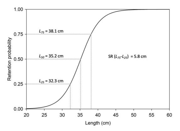
Figure 12. Example of a West Coast groundfish bottom trawl logistic selection curve for Dover sole depicting the model parameters  $L_{50}$  and SR from a 114 mm diamond mesh codend. Data source: Paper IV.
