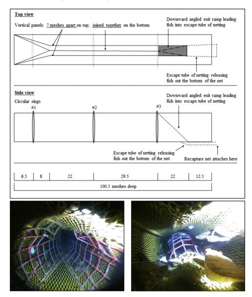
Fig. 1. Schematic diagram of the Pacific halibut flexible sorting grid excluder tested (top); aft view of the forward portion of the excluder where fish enter and encounter the device (bottom left); forward view of the downward-angled exit ramp with fish moving aft toward the codend (bottom right).
