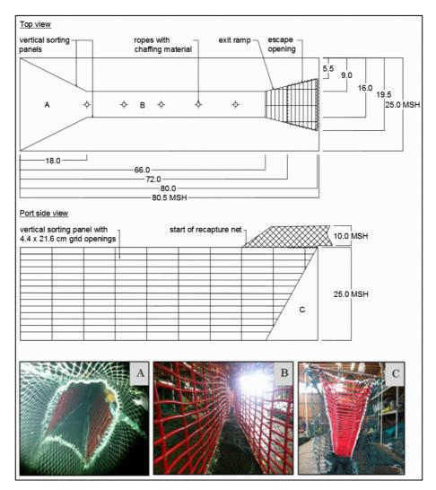
**Figure 14**. Schematic diagram of the sorting grid tested in Paper II (top); aft view of the forward portion of the gear where fish enter and encounter the device (image A); aft view from inside of the BRD (image B); fore view of the upward-angled exit ramp (image C). MSH = meshes. Note: schematic diagram is not drawn to scale. Source: Paper II.
