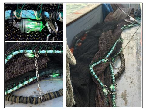
**Figure 8**. Images of artificial illumination placed along the fishing line of an ocean shrimp trawl as a technique to reduce fish bycatch. Source: Hannah et al. (2015).
