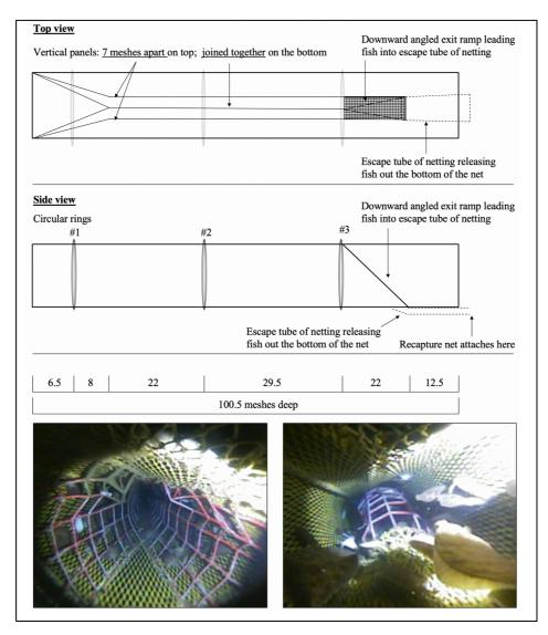
**Figure 13**. Schematic diagram of the Pacific halibut sorting grid BRD tested in Paper I (top); aft view of the forward portion of the excluder where fish enter and encounter the device (bottom left); forward view of the downward-angled exit ramp with fish moving aft toward the codend (bottom right). Source: Paper I.
