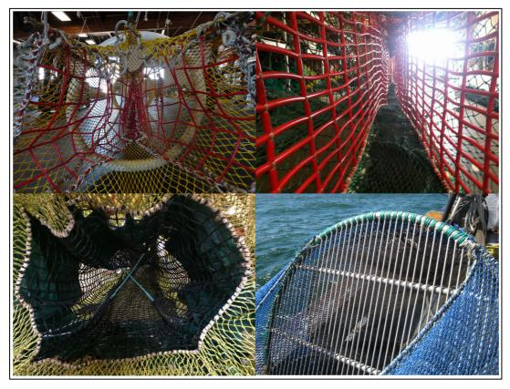
**Figure 4**. Example of sorting grid BRDs designed to reduce bycatch of Pacific halibut (top left image) and roundfishes (top right image) in the West Coast groundfish bottom trawl fishery, rockfishes in the Pacific hake fishery (bottom left image), and fish in the ocean shrimp fishery (bottom right image).
