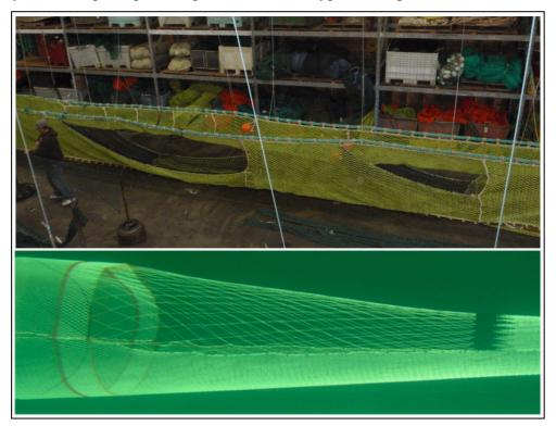
**Figure 7**. Open escape window BRD designed to reduce Chinook salmon bycatch in the Pacific hake fishery (top image; Source: Lomeli and Wakefield [2012]); example of a large mesh panel BRD (bottom image; Source: Krag et al. [2014]).
