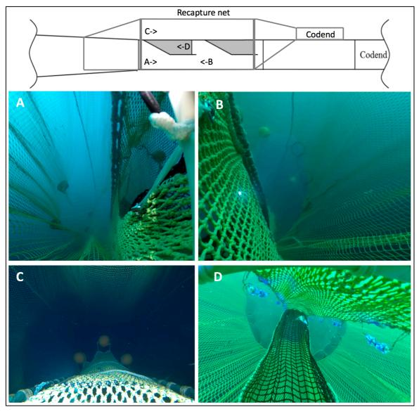
**Figure 19**. Schematic diagram and images under ambient light examining the recapture net over the BRD in Experiment 2 presented in Paper VIII. A = port-side aft view from outside of the BRD; B = starboard-side forward view from outside of the BRD; C = top panel aft view from outside the BRD; D = forward view of the forward set of escape windows from within the BRD. Note: diagram not to scale. Source: Paper VIII.
