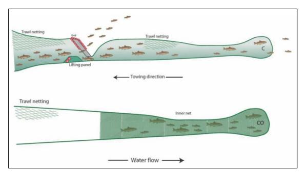
**Figure 11**. Example of the paired-gear method for collecting absolute size selectivity data. Source: Grimaldo et al. (2016).
