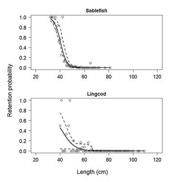
**Fig. 7.** Mean selectivity curves showing the probability of retaining sablefish and lingcod by length in the trawl codend. Circles are the experimental data; solid lines are the modeled value; dashed lines are upper and lower 95% confidence interval limits.
