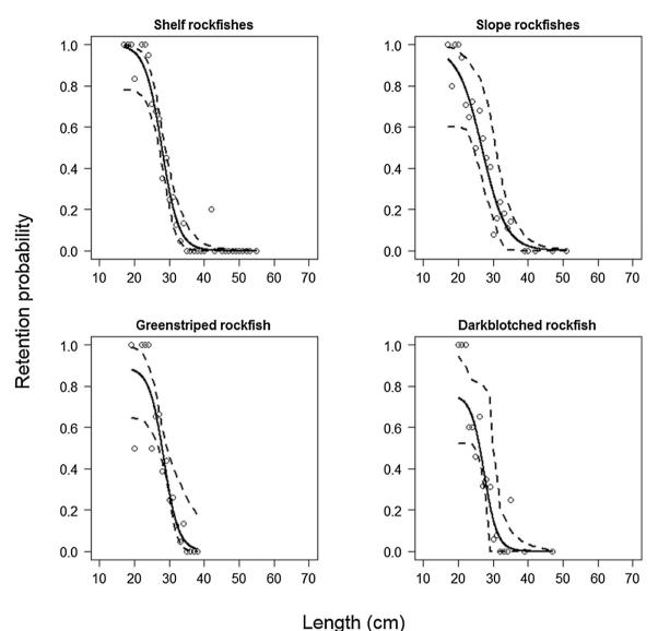
Fig. 6. Mean selectivity curves showing the probability of retaining shelf and slope rockfishes, greenstriped rockfish, and darkblotched rockfish by length in the trawl codend. Circles are the experimental data; solid lines are the modeled value; dashed lines are upper and lower 95% confidence interval limits.
