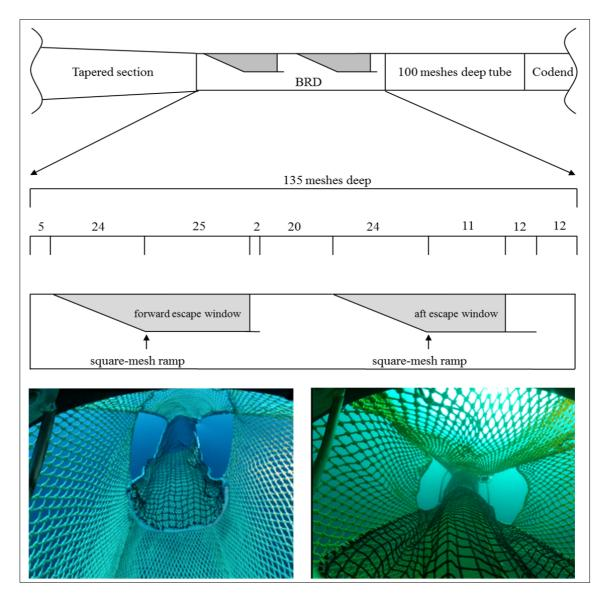
**Figure 18**. Schematic diagram of the open escape window BRD used in Paper VIII (top); forward view of the forward set of escape windows under ambient light (left image); forward view of the aft set of escape windows under ambient light (right image). Note: diagram not to scale. Source: Paper VIII.
