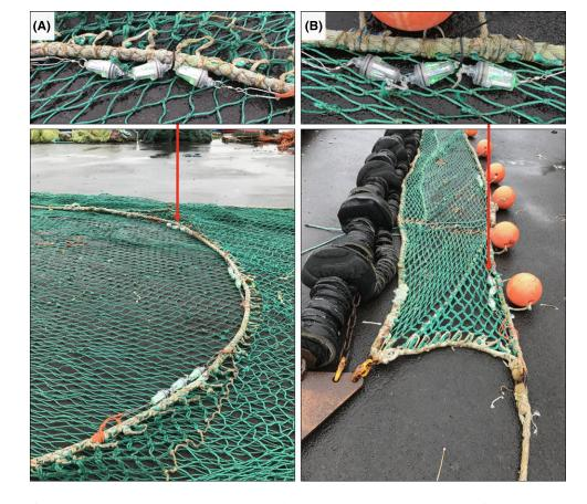
FIGURE 1. Images of an LED cluster attached (A) near the center of the trawl headrope on the starboard side and (B) along the wing tip on the port side, and their orientations.
