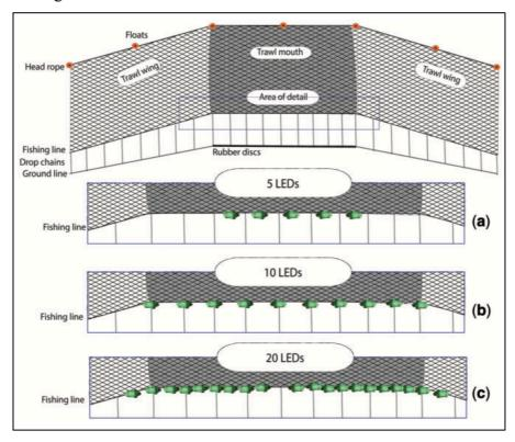
**Figure 17**. Schematic of an ocean shrimp trawl viewed from the front (top image) and diagrams depicting the placement and orientation of the LEDs along the trawl fishing line for the 5 (a), 10 (b), and 20 LED (c) configurations. Note: diagram not to scale. Source: Paper VI.
