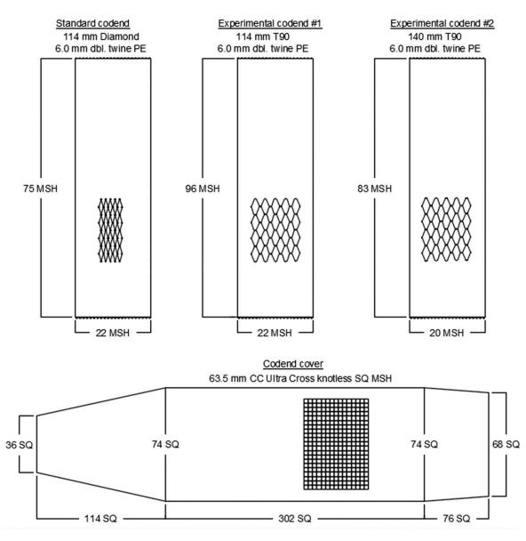
FIGURE 1. Schematic diagram depicting a top-panel view of the cod ends and the cod end cover used in evaluating the cod end types for the West Coast groundfish bottom trawl fishery. Diamond mesh (DM) and T90 mesh sizes are nominal stretched measurements between knots (MSH = mesh; dbl. = double twine; PE = polyethylene; CC = center-to-center mesh measurement; SQ = square). Diagram is not drawn to scale.
