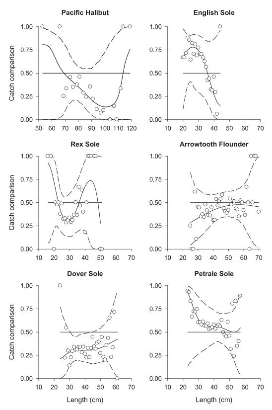
FIGURE 3. Mean catch comparison curves for flatfishes per size-class. Circles denote the experimental data; solid curves are the modeled values; dashed lines represent the 95% confidence interval limits; horizontal lines depict the baseline catch comparison rate of 0.5, indicating equal catch rates between the treatment and control trawls.
