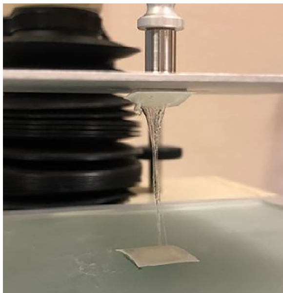
Fig. 8. Picture illustrating the over-plasticised effect of wetting a Soluplus® single polymer film.
