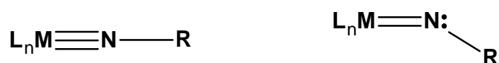
Figure 21. The linear (left) and bent (right) bonding arrangement of terminal imido ligands.
