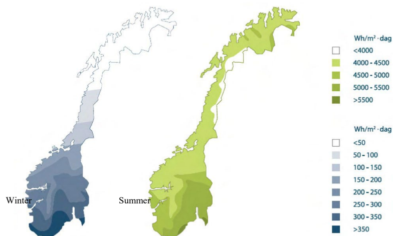
Figure 1. Solar irradiation on a horizontal surface in Norway for winter and summer [5].
