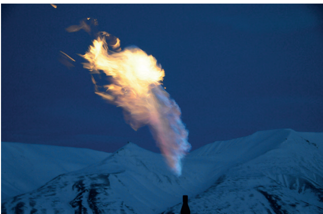
Figure 9. Flared thermogenic gas from open hole at 648–701 m depth, well DH5R. Stable semi-dry gas, i.e., 95% methane was produced at a stable rate of 1500 Sm 3 /day, see Ohm et al. (2019) for details.
