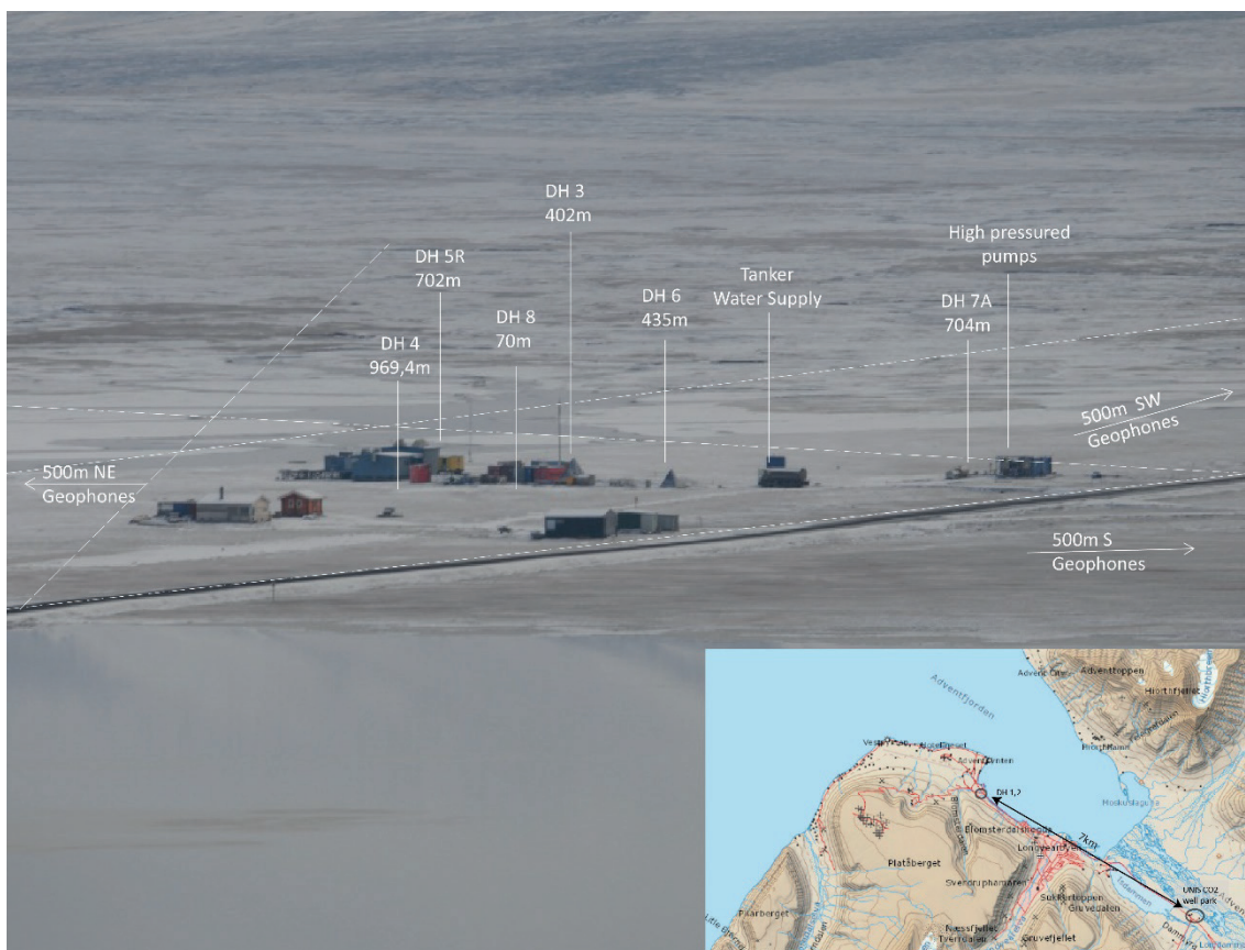
Figure 1. Overview of the UNIS CO 2 Lab well park in Adventdalen, south-east of Longyearbyen. The inset map shows the UNIS CO 2 Lab well park location, as well as the location of the DH1 and DH2 boreholes near Longyearbyen airport. All publications in this appendix are partly based on data from these boreholes. The numbers beneath the well numbers indicate s total drilled depth (TD) of each borehole. All wells apart from DH3 are now plugged and abandoned (P&A). In addition, temporary shallow geophones were installed within a 1 km radius of the UNIS CO 2 Lab well park during the operational phase. Stippled lines shows position for some of the conventional 2D seismic lines acquired in this area.
