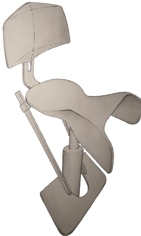
Figure 23 Watercolor sketch of the working chair. The strap fixating the position of the footrest and the lower part of the undercarriage, including wheels, are not included in the sketch.
