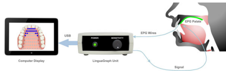
Figure 3.4: Diagram for an Electropalatography system in use, source (Rose Medical Solutions, 2019a).
